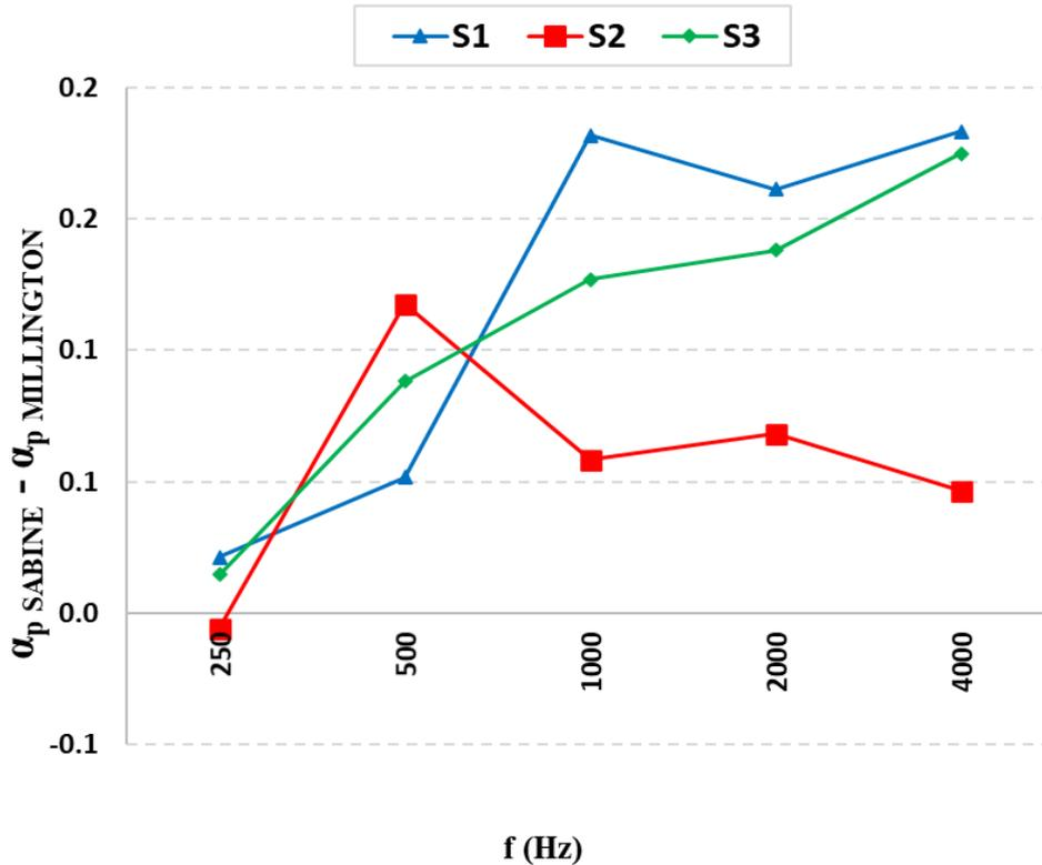
Figure 2 – Differences between Sabine and Millington-Sette sound absorption coefficients for samples S1, S2 and S3: (a)  $\alpha_s$ ; (b)  $\alpha_p$
