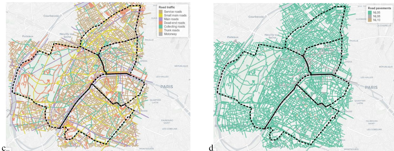
Figure 2 – Main input data for NoiseModelling from OSM (example of a part of Paris city noise map): a) buildings, b) ground absorption, c) road traffic, d) road pavements.
