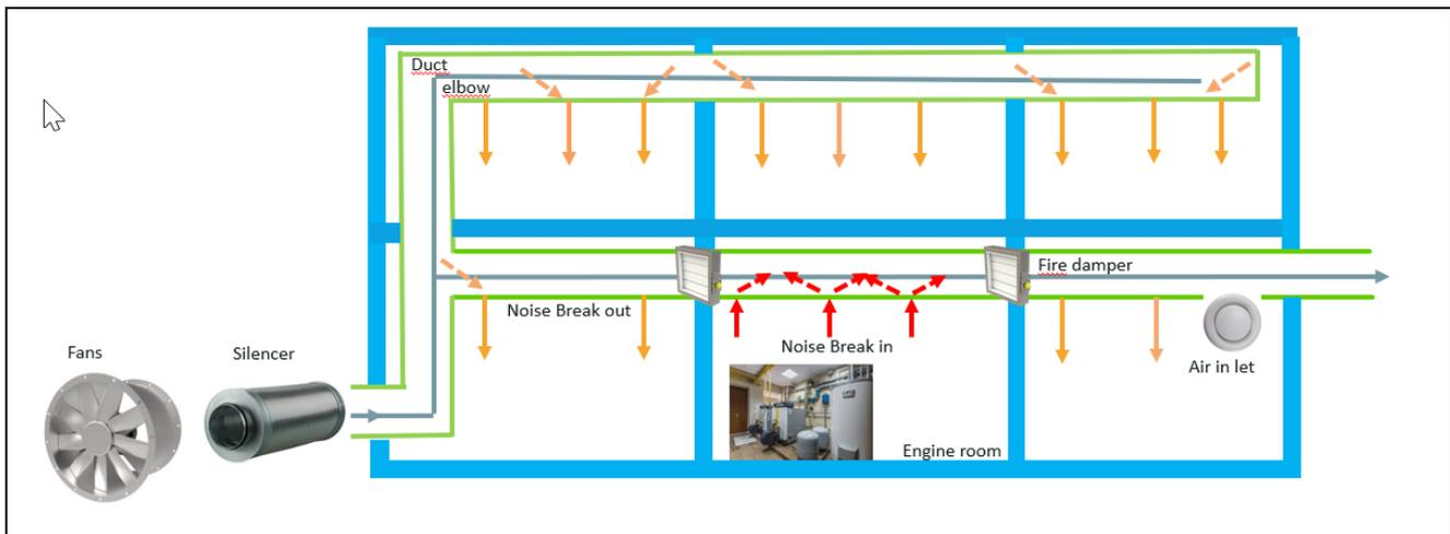
Figure 1 – Scheme of impact of background noise due to operating noise of extraction and ventilation duct.
