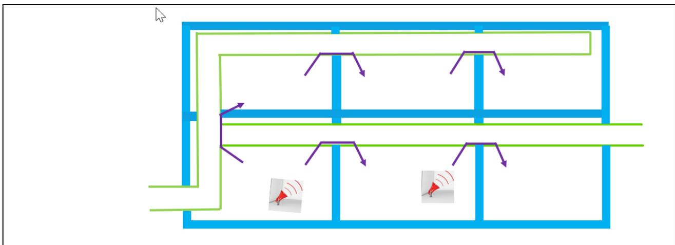
Figure 2 – Scheme of lateral flanking sound transmission due to duct penetration of the compartment boundaries.
