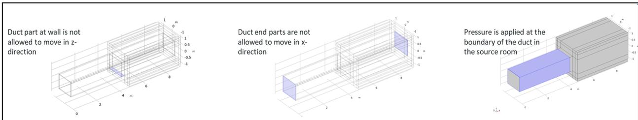
Figure 5 – Geometry and boundary conditions of the duct model
