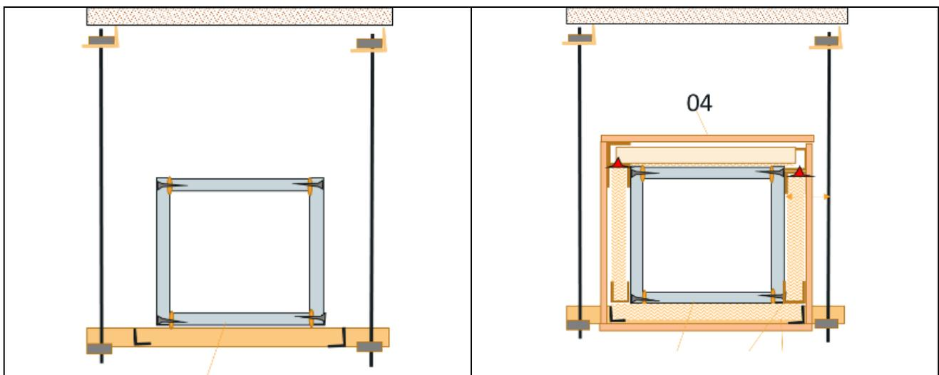
Figure 4 – Tested configuration – Left: calcium silicate duct with typical structure of assembly – Right: calcium silicate duct with additional acoustic lining.
