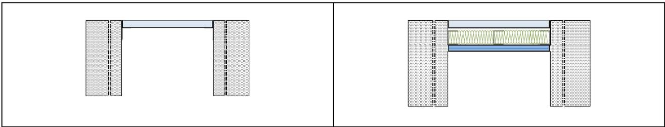
Figure 3 – Drawing of tests configuration – Left: single calcium silicate duct panel – Right: acoustic lining on calcium silicate panel.
