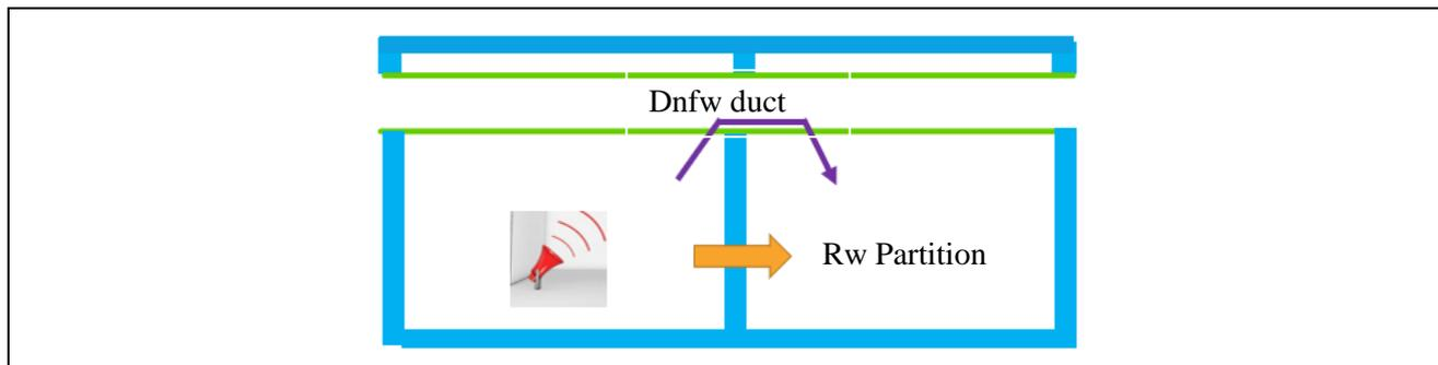
Figure 7– Scheme of the direct sound transmission of the separating element and the lateral transmission path of the ventilation duct.
