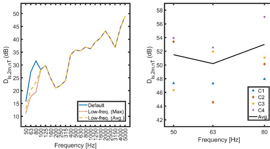
Figure 2: Room R2. Left - Sound insulation (i.e.,  $D_{Is,2m,nT}$ ) derived following the three calculations: default method, standardized low-freq. procedure, and average low-freq. procedure. Right –  $L_2$  measured at each of the four corners as well as the average value for 50, 63 and 80 Hz bands.
