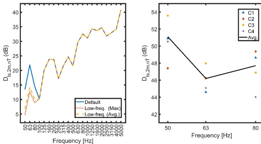
Figure 1: Room R1. Left - Sound insulation (i.e.,  $D_{Is,2m,nT}$ ) derived following the three calculations: default method, standardized low-freq. procedure, and average low-freq. procedure. Right -  $L_2$  measured at each of the four corners as well as the average value for 50, 63 and 80 Hz bands.
