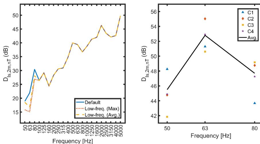
Figure 3: Room R3. Left - Sound insulation (i.e.,  $D_{Is,2m,nT}$ ) derived following the three calculations: default method, standardized low-freq. procedure, and average low-freq. procedure. Right –  $L_2$  measured at each of the four corners as well as the average value for 50, 63 and 80 Hz bands.
