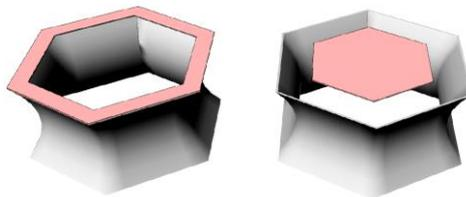
Figure 2 – Two approaches for partially covering the ceiling, donut style and suspended central canopy
