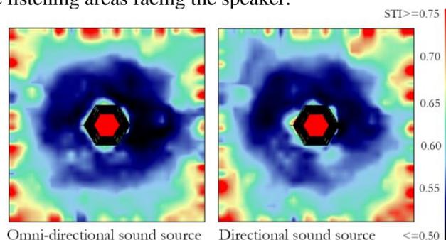
Figure 1– STI maps with directional vs. omnidirectional sound source
