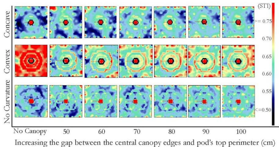
Figure 3 – Matrix A-1, Exploring STI maps of three types of the pods with suspended central canopy of various sizes
