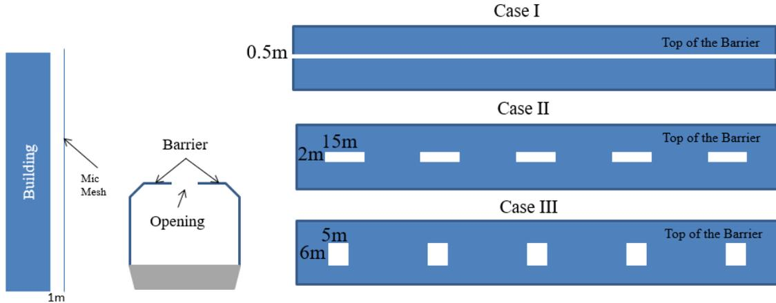
Fig.3 Schematic diagram of three types of openings
