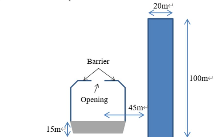
Fig.2 The schematic diagram of the overhead subway
