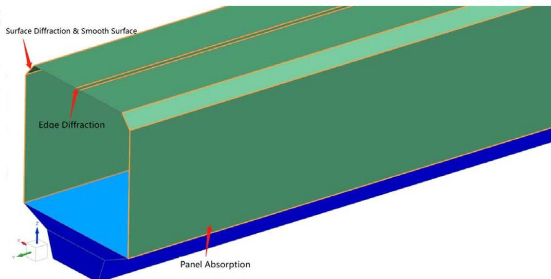
Fig.9 Schematic diagram of sound barrier surface and edge setting
