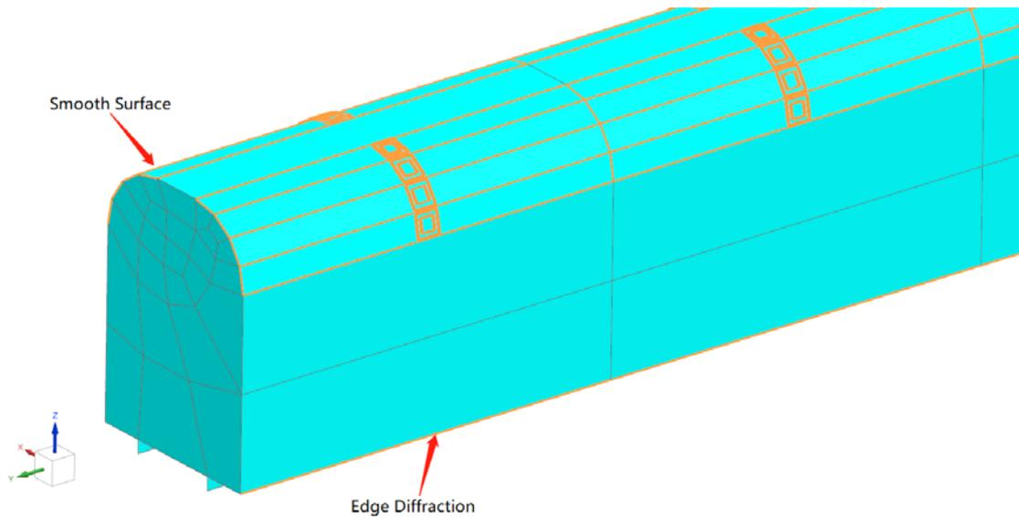
Fig.8 Schematic diagram of train surface and edge setting
