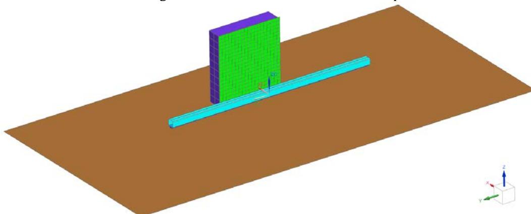
Fig.5 Acoustics Mesh of the Barrier
