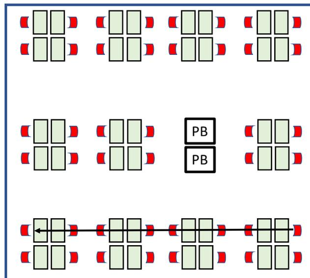
Figure 2 - Principal workstation layout of the open-plan office demonstrated in Sec. 4. The floor dimensions were 14x14 m. The number of workstations was 44. PB is a phone booth. Measurement path is indicated by black line.
