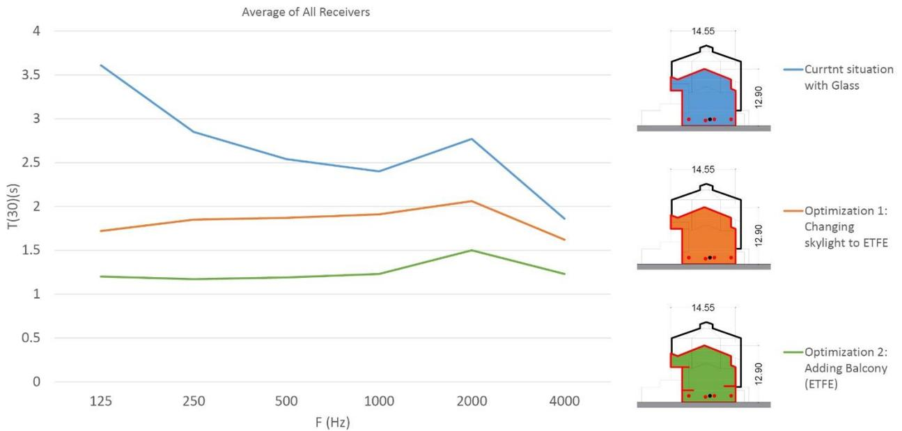
Figure 6 –  $T_{30}$  comparison between current situation and optimizations at 6 octave bands
