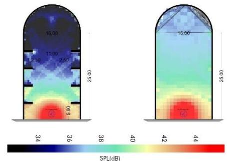
Figure 5 – Section of Sound Pressure level(SPL) comparison at 1000Hz
