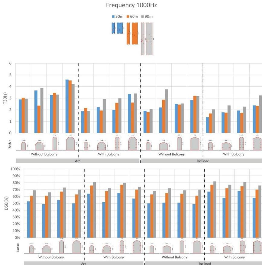
Figure 3 – Length comparison for  $T_{30}$  and  $D_{50}$  at 1000Hz
