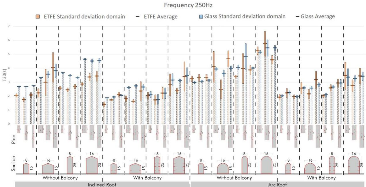
Figure 2 – Material Comparison  $T_{30}$  (250Hz)
