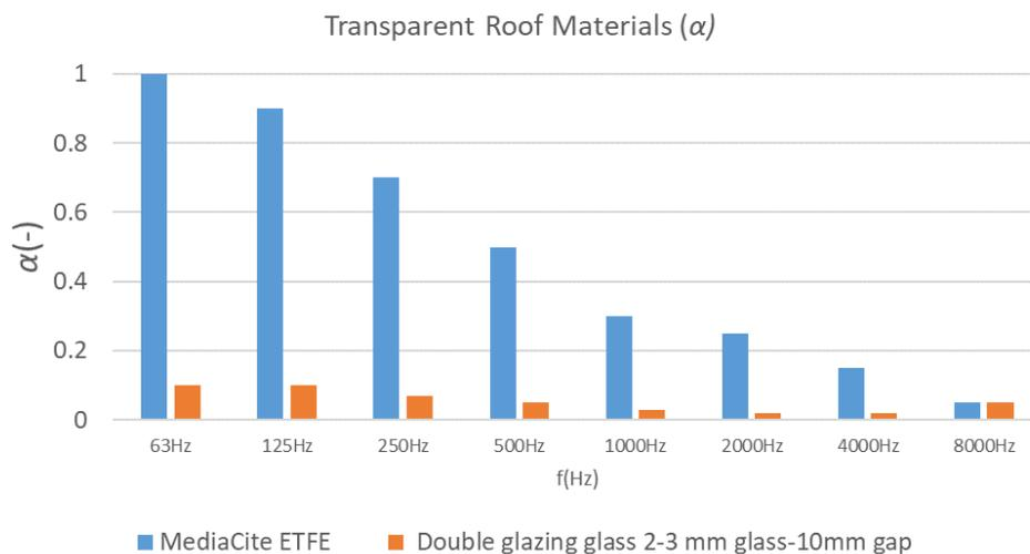
Figure 1 – Sound Absorption Coefficient ( $\alpha$ (-)) of the ETFE and glass
