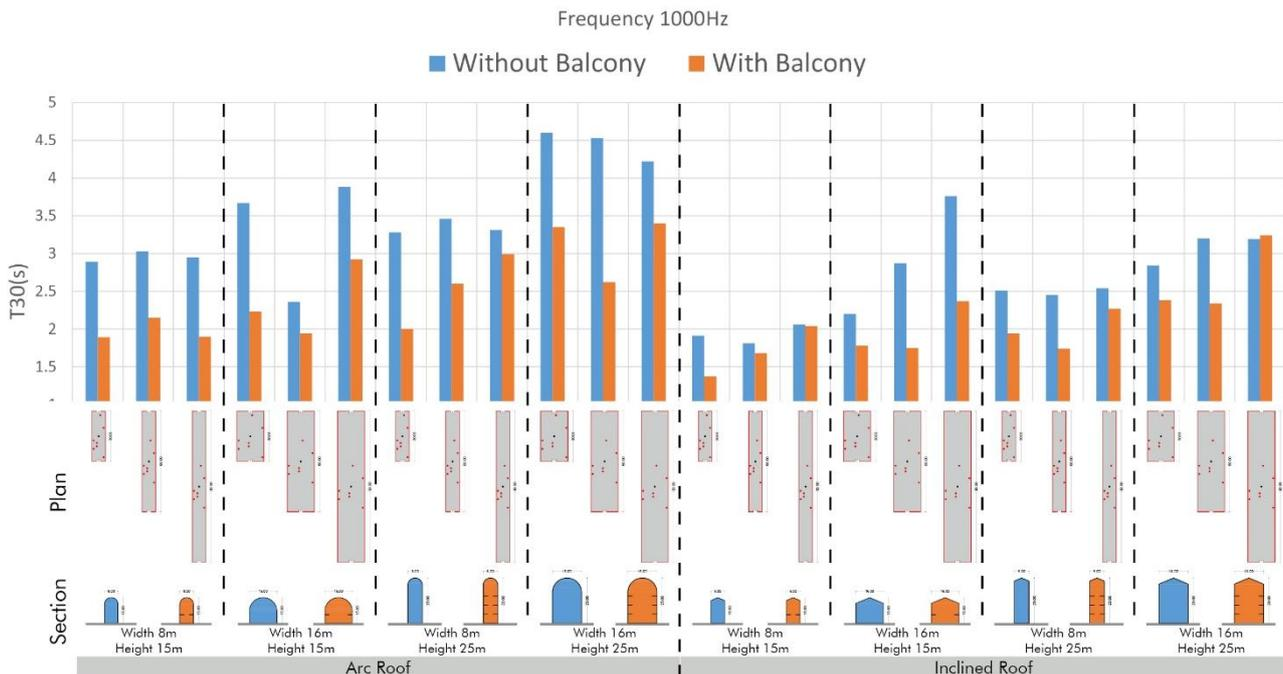
Figure 4 – Effect of Balconies in  $T_{30}$  at 1000Hz
