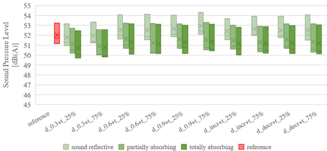
Figure 5 - Variation of A-weighted SPL for courtyard receivers (i.e. at the ground level of building B) resulting from the different material and geometric configurations tested.
