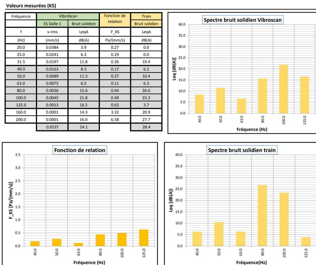
Figure 7 - Example of the calculation of ground-borne noise immissions (KS) starting from measured values. The green columns refer to measured data and allow to calculate the  $F_{KS}$  coefficient. From  $F_{KS}$  coefficient and train emissions data (not shown here) it is possible to determine train ground-borne noise immissions.
