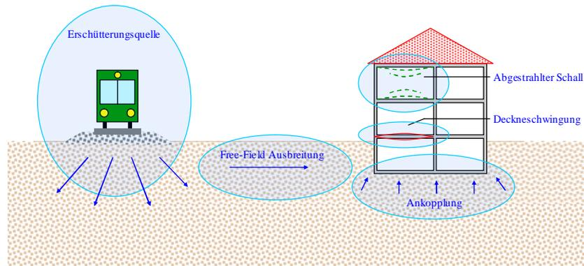
Figure 2 – Propagation of vibrations from the railway line to nearby buildings [5]
