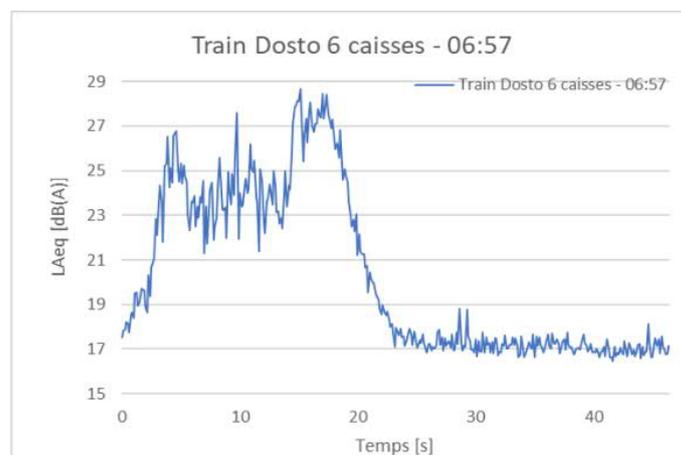
Figure 8 - Example of measured ground-borne noise on a section with LVT-HA
