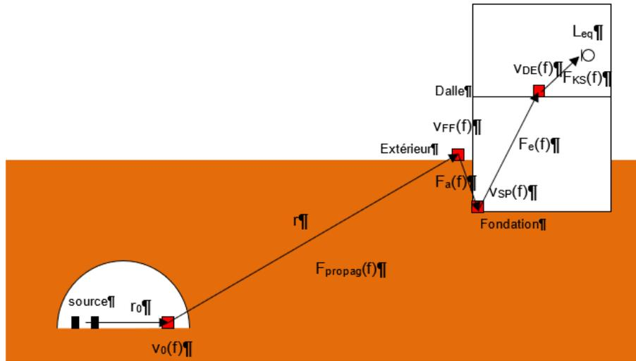
Figure 6 - Schematic representation of the measurement setup
