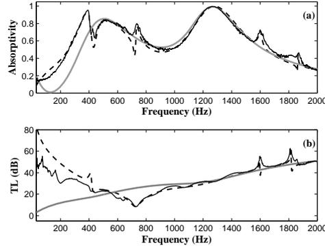
Figure 4 - Measured (black solid) absorptivity (a) and TL (b) for the MPP partition and comparison against predictions by the transfer approach (gray solid) and by a modal formulation (black dashed).
