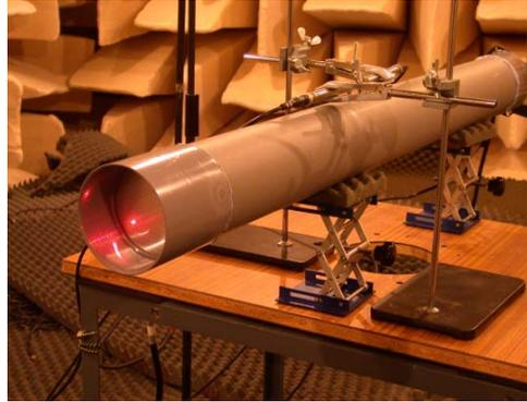
Figure 2- Photograph of the transparent back face of the MPPA for determination of its vibrating response.
