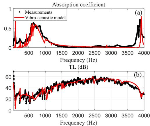
Figure 8 - Absorption coefficient (a) and TL (b) of a clamped micro-perforated partition under normal incidence: modal approach (red solid) and experiment (black solid).
