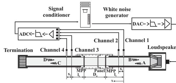
Figure 3- Experimental facility to measure sound absorption and transmission under normal incidence.
