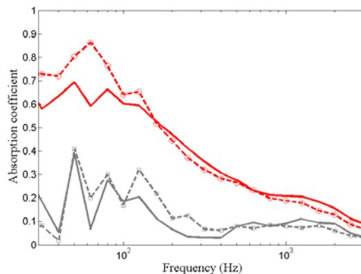
Figure 12 - Third-octave averaged absorption curves for a number of partitions undergoing a TBL excitation: plain front panel (solid grey: calculated; dashed grey: measured), micro-perforated front panel (solid red: calculated; dashed red: measured).
