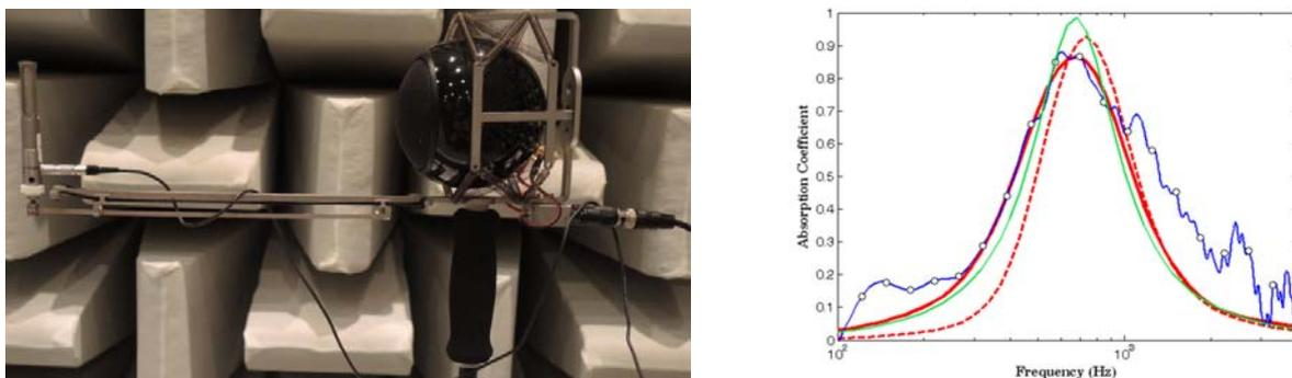
Figure 6 - Photograph of the impedance gun for *in-situ* measurement of the absorption properties (left) and normal incidence absorption coefficient of the input impedance of a fiberglass material shielded by a thin MPP (right): comparison between  $p$ - $v$  free-field measurements (blue) and predictions from the Miki-Delany-Bazley (green) and from an anisotropic (red-dashed) and fully anisotropic model (solid red) [13].
