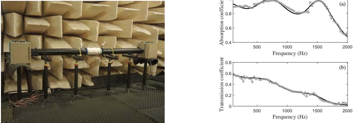
Figure 5 - Photograph of the impedance transmission tube by the two-source method (left) and absorption (a) and transmission (b) coefficients of a multi-layer partition made up of three MPPs under normal incidence: comparison between Kundt tube measurements (gray dotted) and modal approach (black solid).
