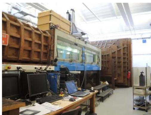
Figure 9 - Overall view of the low-speed wind-tunnel facility equipped to measure the TL and absorption coefficient of TBL-excited MPP partitions flush-mounted over the top wall of the test section.
