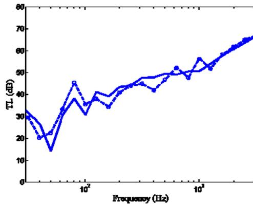
Figure 11 - Third-octave averaged TL curves for the micro-perforated partition under a TBL excitation: measured (blue dashed) and predicted (blue solid).
