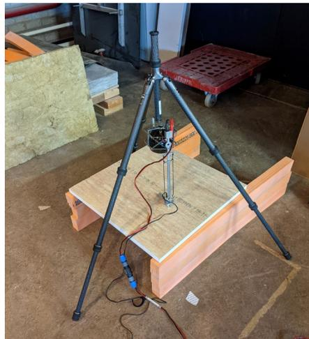
Figure 2 – Picture of the experimental validation setup. The sample of material B is mounted on rubber bars to create a 240 mm air gap between the sample and the concrete.
