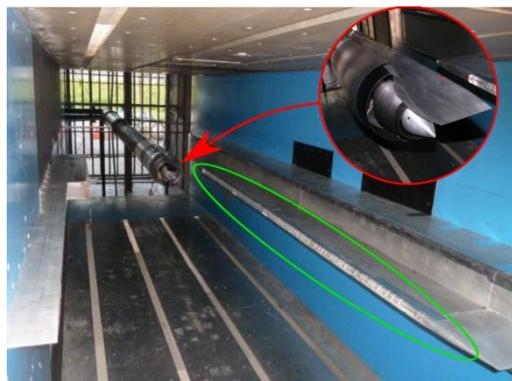
Figure 2 : Overview of the test section. The red zone is a zoom of the nozzle. The green zone shows the rail where the microphones are flush-mounted.
