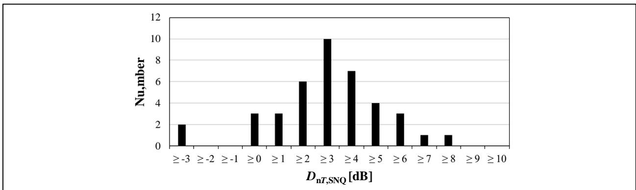
Figure 4 – Distribution of the differences of the single-number quantities  $D_{nT,SNQ}$ .
