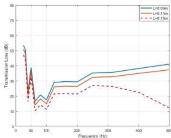
Figure 5. Impact of the size of the mullion on the Transmission Loss
