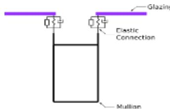
Figure 9. Schematic of the mullion/glazing connection
