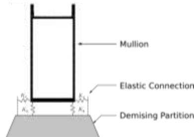
Figure 6. Schematic of the elastic boundary condition between the mullion and the demising partition
