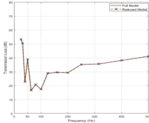
Figure 12. Comparison of the transmission between a reduced mullion element and the full model
