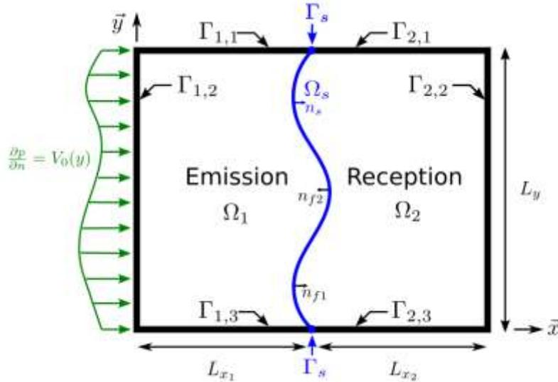
Figure 1. Schematic of a vibro-acoustic model
