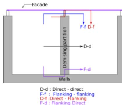
Figure 3. Schematic of the flanking paths between two rooms
