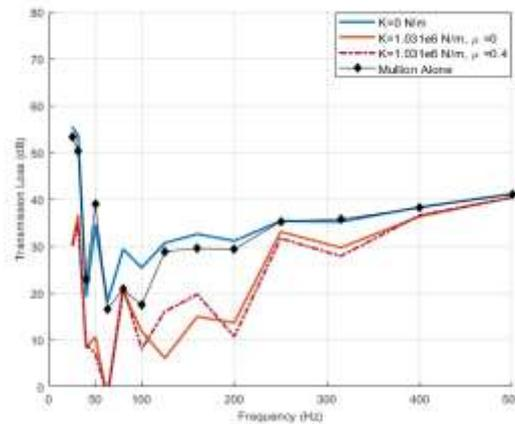
Figure 10. Transmission Loss for the Mullion/Glazing system
