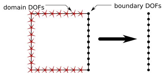
Figure 11. Schematic of the condensation
