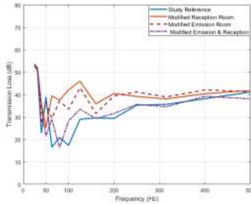
Figure 8. Impact of the room geometry on the Transmission Loss
