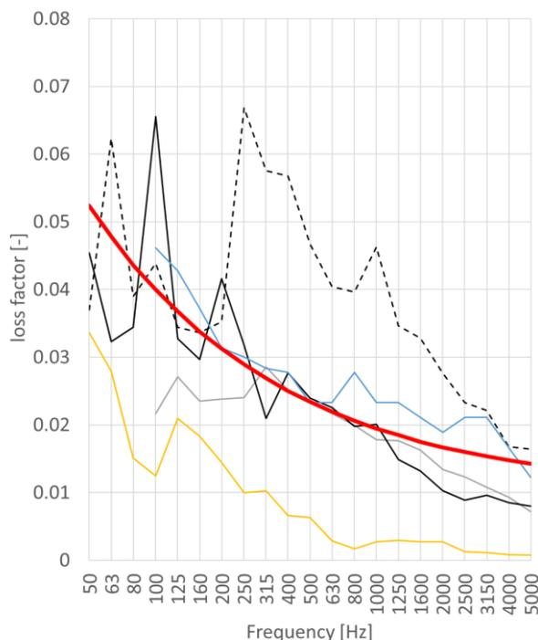
(a) Loss factor measured at 4 laboratories and minimum loss factor required by ISO 10140 (red)
