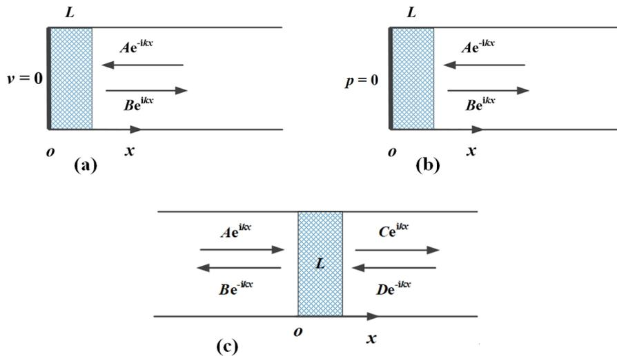
Figure 1: The 1D scattering problem of a plane wave by a composite material: (a) Symmetric reflection problem; (b) Anti-symmetric reflection problem; (c) Symmetric transmission problem.
