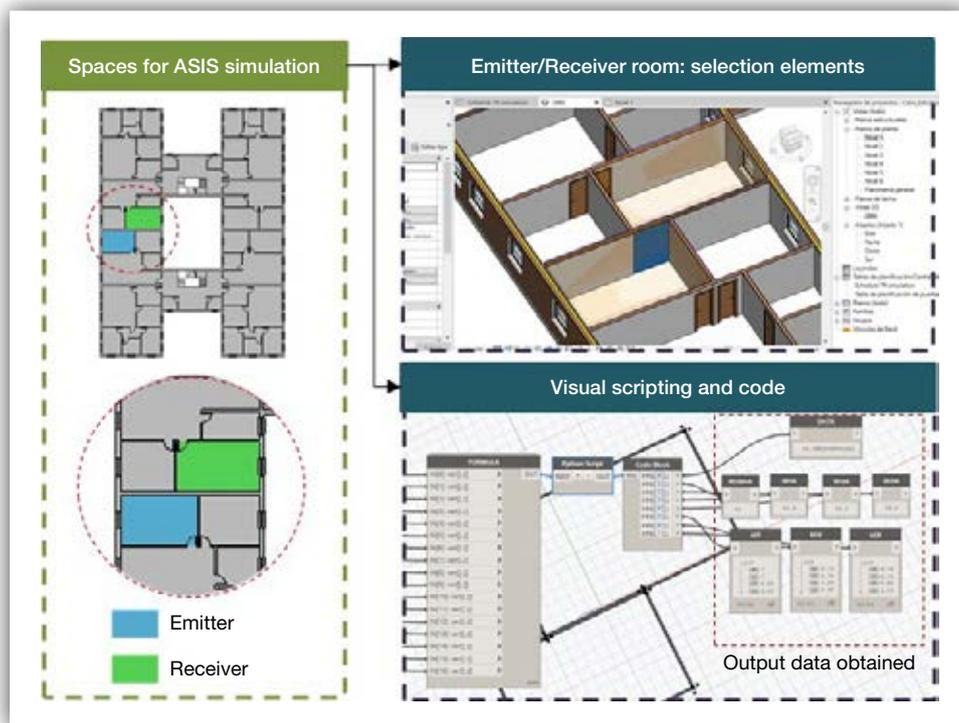
Figure 7. Process for element selection to perform ASIS simulation.
