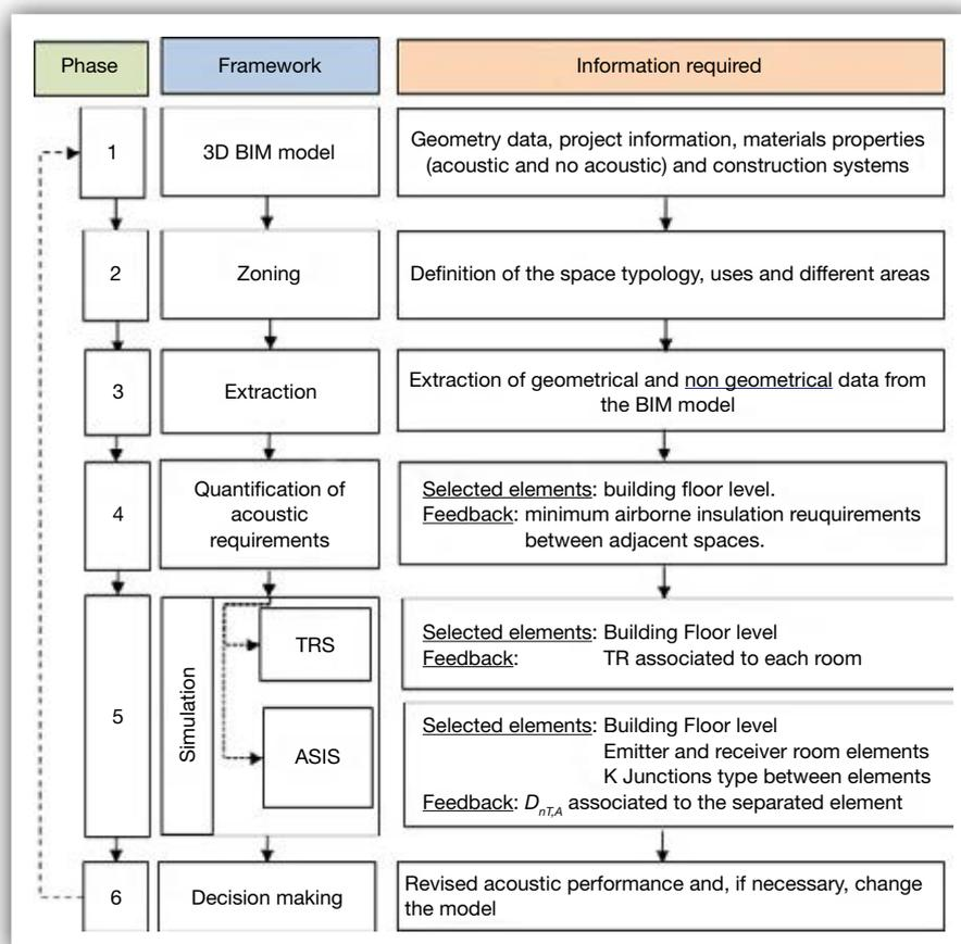
Figure 3. Diagram of the proposed workflow process.
