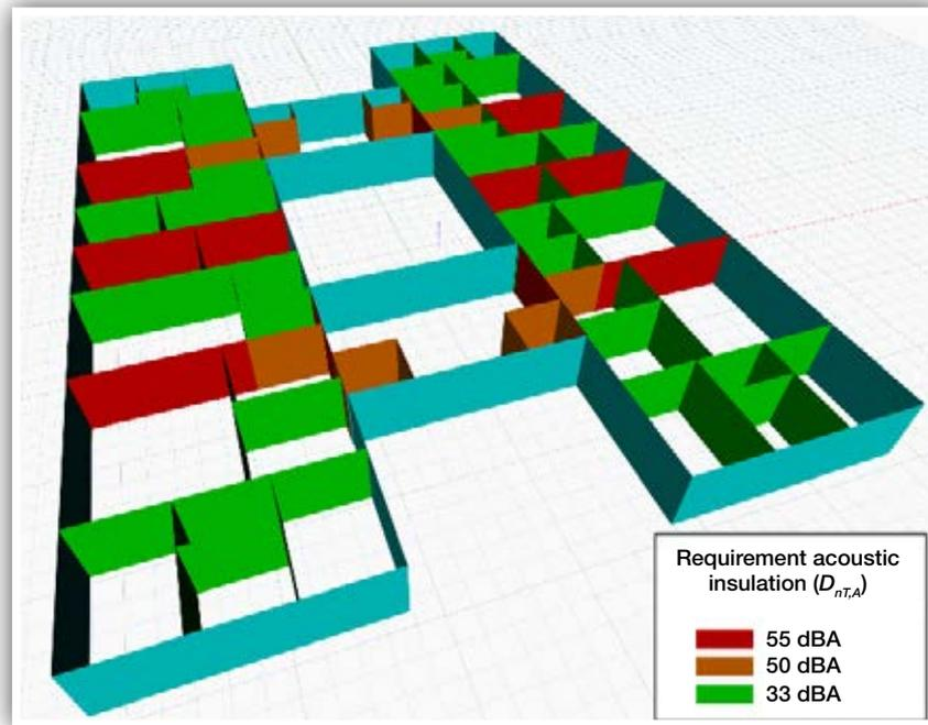
Figure 5. Visualization of the requirements of acoustic insulation to airborne noise between rooms.
