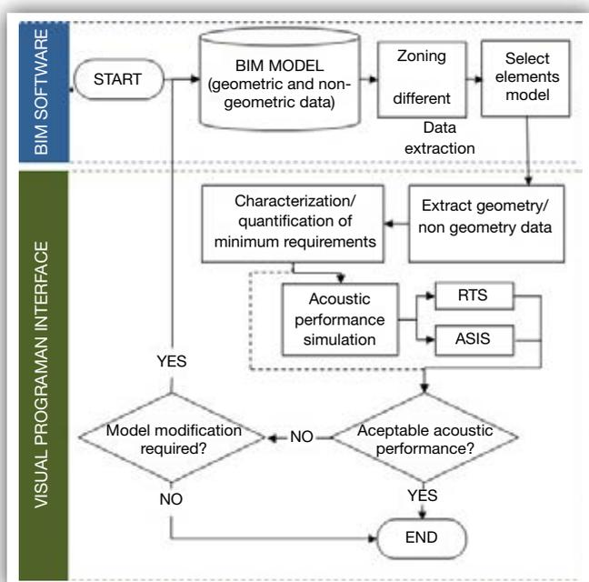
Figure 2. Diagram of the acoustic simulation process and developed software.
