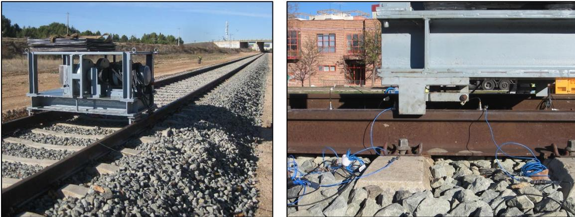
Figure 5 – Excitation device placed in the ballasted railway track under study in Aranda de Duero (Burgos).
