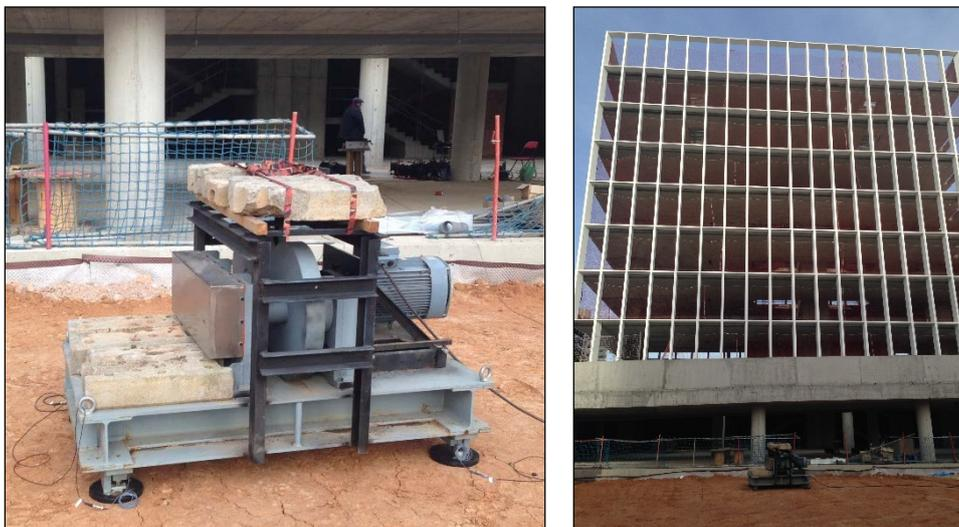
Figure 3 – Excitation device placed in the surface of the nearby ground of a building in Sant Adrià del Besòs (Barcelona).
