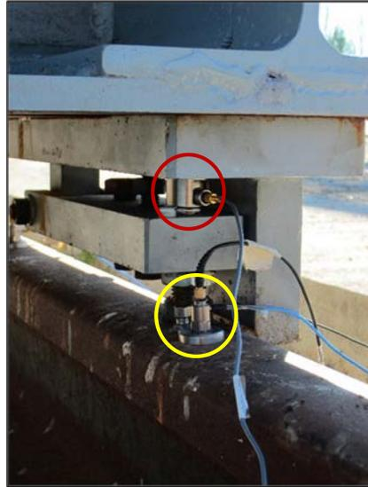
Figure 2 – Excitation device supporting system for one of the four supports and example of transducers setup (Force transducer denoted in red and accelerometers in the rail denoted in yellow).
