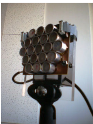
Figure 3. Image and pattern diagram of the ultrasound loudspeaker array.
