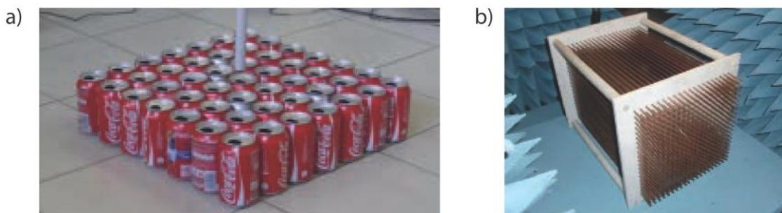
Figure 1 – Two examples of locally resonant metamaterials: (a) an acoustic example based on Helmholtz resonators (the soda cans), and (b) a microwave one based on half-wavelength-long copper wires.
