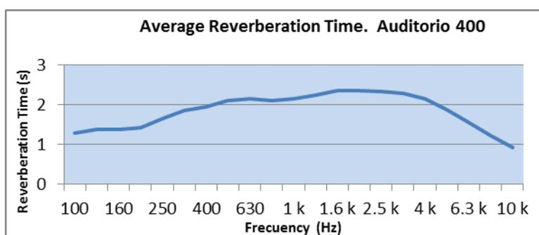
Figure 8- Reverberation Time vs. frequency
