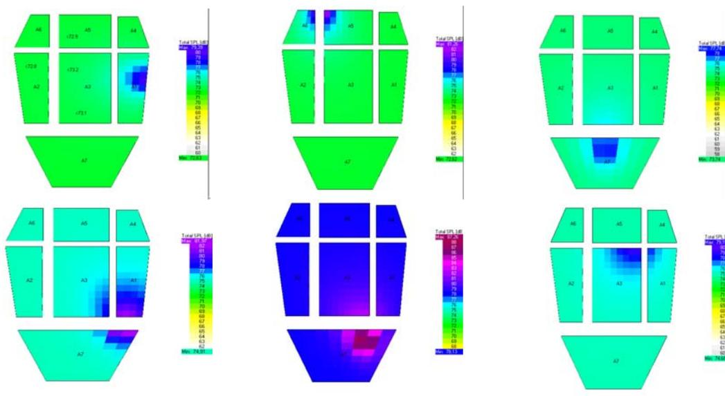
Figure 7.- Examples of SPL for a single speaker
