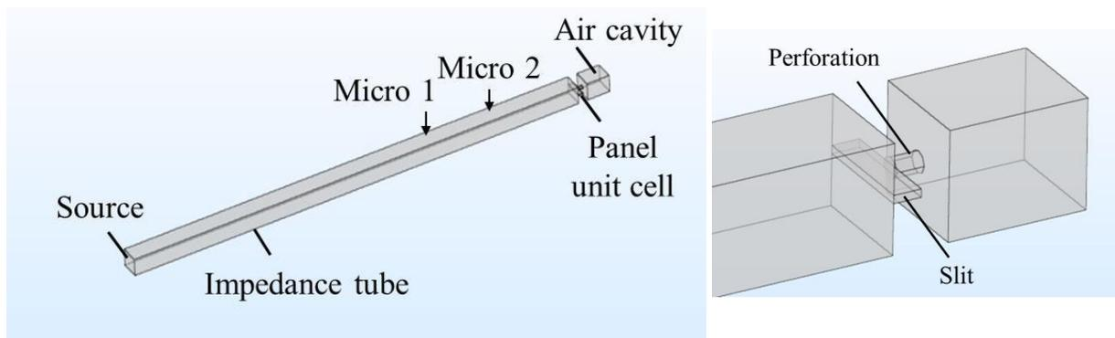
Figure 3 - Numerical model of the impedance tube setup. (Left) General view. (Right) Detailed view.
