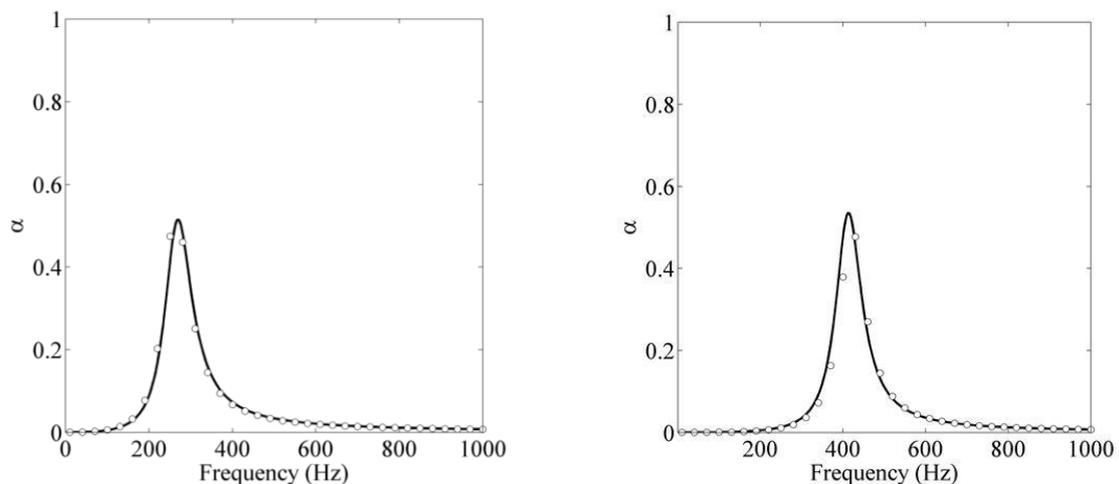
Figure 4 - Normal incidence sound absorption coefficient for the configurations (Left) GAP1 and (Right) GAP2. Solid line, TMM model; circles, FEM model.
