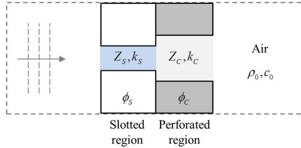
Figure 2 - Cell geometry of a grooved acoustic panel.
