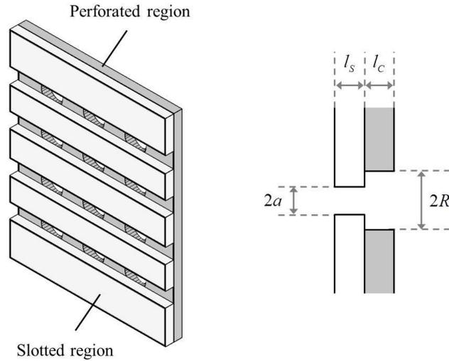
Figure 1 - Schematic representation of a grooved acoustic panel. (Left) General view. (Right) Detailed view.
