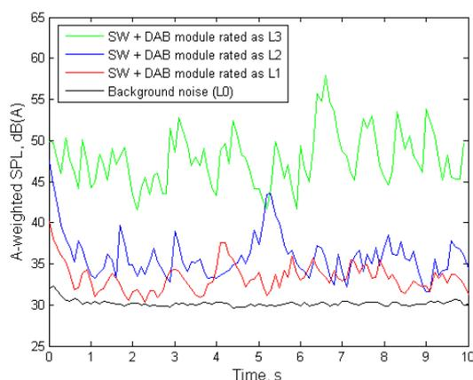
Figure 4 – A-weighted sound pressure level versus time measured for three different steering wheel plus DAB module assemblies producing rattle noise evaluated with different ratios.
