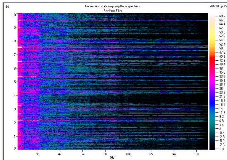
Figure 5 – Spectrogram measured for one of the steering wheel plus DAB module assembly that generated rattle noise rated as L3.
