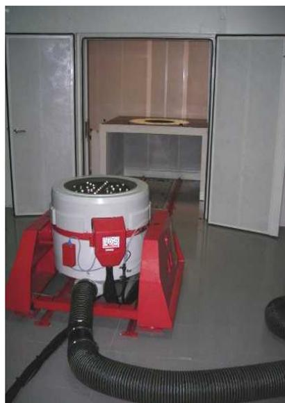
Figure 1 – Facility used during the test: An electrodynamic shaker was used for the vibration excitation. This was installed inside an acoustic enclosure to reduce the noise from the shaker inside the chamber. The measurements were carried out inside the CTAG anechoic chamber.
