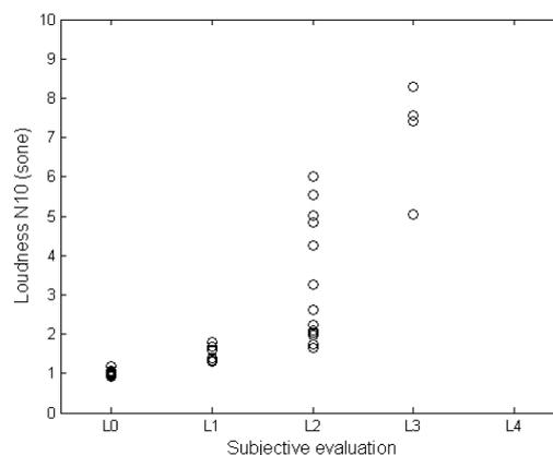
Figure 6 – Comparison between the measured statistical loudness (N10) and the subjective evaluation for the different tests samples.
