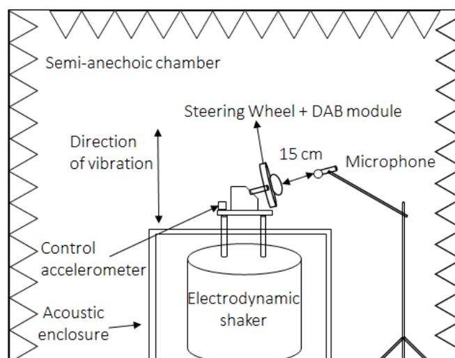
Figure 2 – Test set-up used for the application of the vibration profile in the Z direction.
