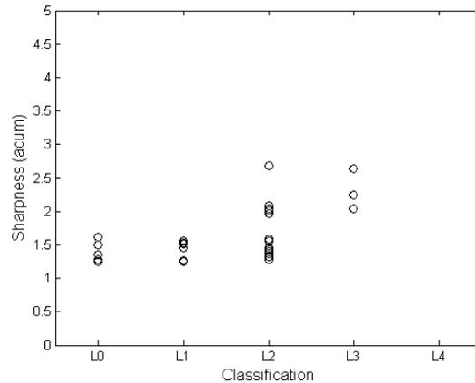
Figure 8 – Comparison between the measured statistical sharpness (N10) and the subjective evaluation for the different tests samples.
