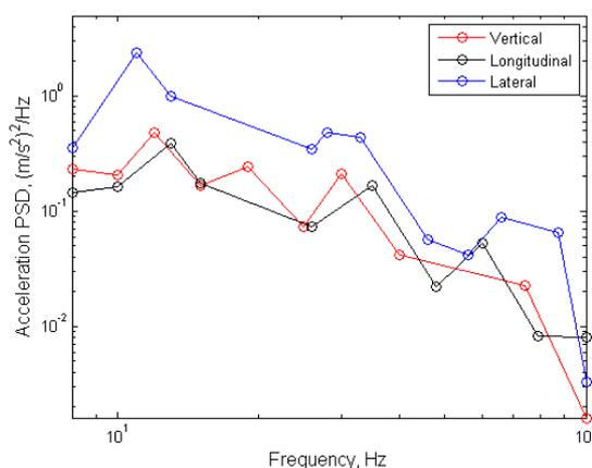
Figure 3 – Random vibration profiles used for exciting the steering wheels during the noise evaluation. Profiles according to the General Specification GMW 14096 [9].
