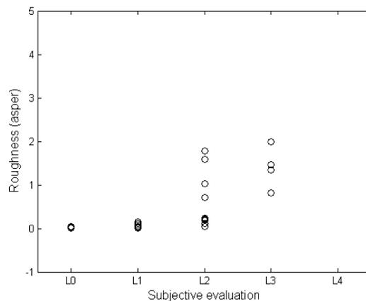
Figure 9 – Comparison between the subjective ration and the measured roughness.
