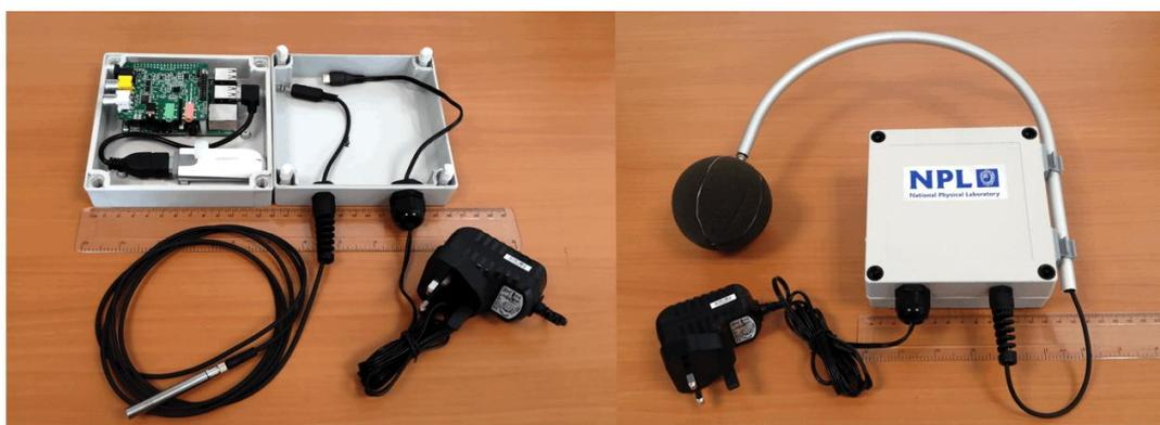
Figure 1: NPL's Raspberry Pi based wireless sensor network's measurement station.
