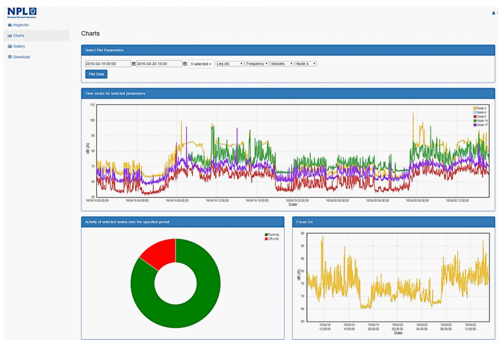
Figure 6: Screenshot of the web interface's Chart tab presenting data collected from the railway construction site over the first two days.
