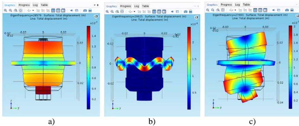
Figure 1 – Different vibration modes of the Langevin type transducer. a) Axial mode (25879 Hz). b) Flexural mode in the flange (29625 Hz). c) Torsional mode (27693 Hz).
