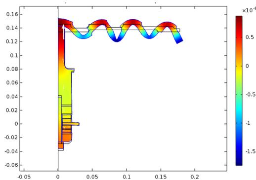
Figure 4 – Vibrational behaviour of the transducer at 24928 Hz.
