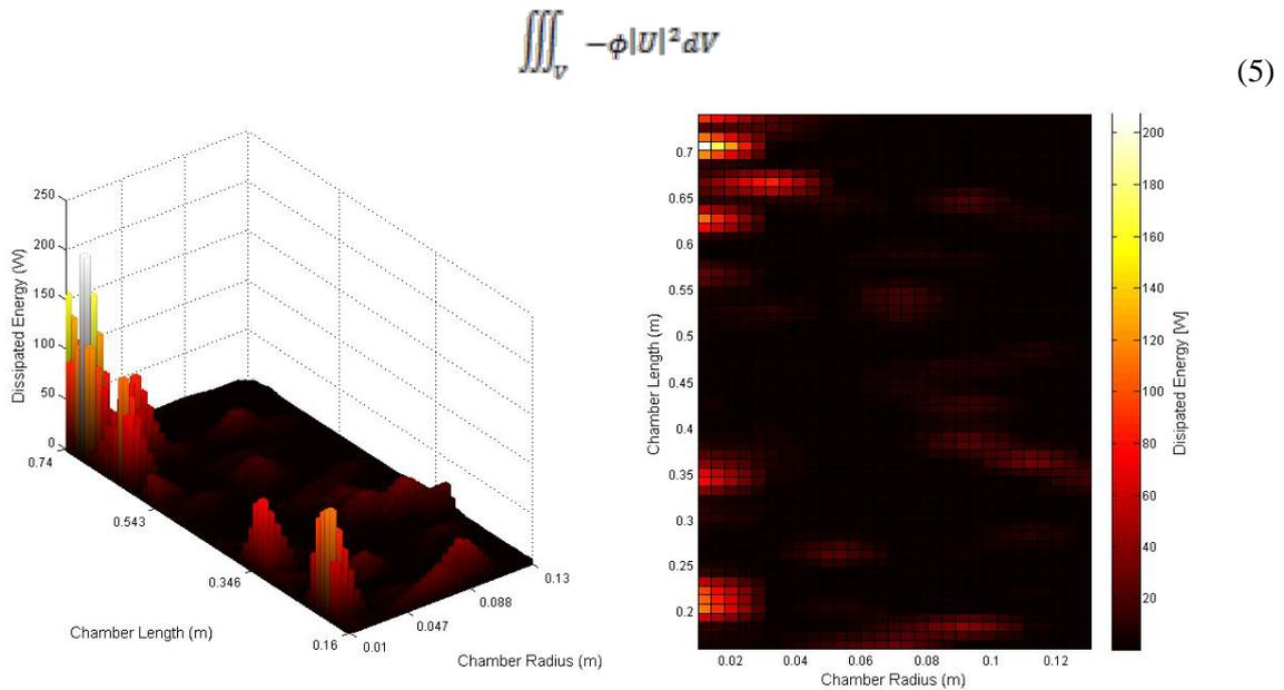
Figure 10 – Map with the dissipated energy inside the potato sample, depending on the sample's location in the drying chamber.
