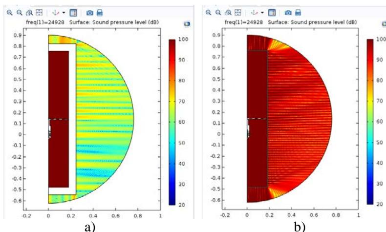
Figure 7 – Acoustic field generated outside the chamber with (a) thick or (b) thin chamber walls.
