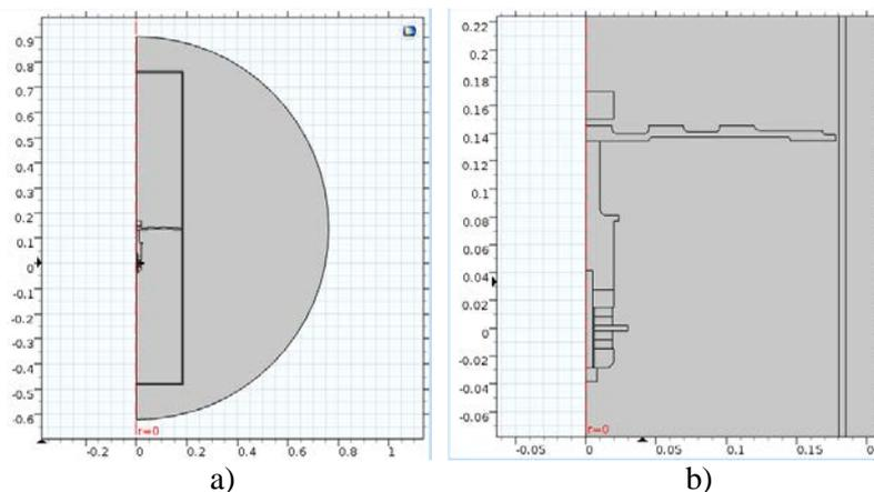
Figure 9 – a) Model of the system. b) Detail with the potato sample and the circular stepped plate transducer.
