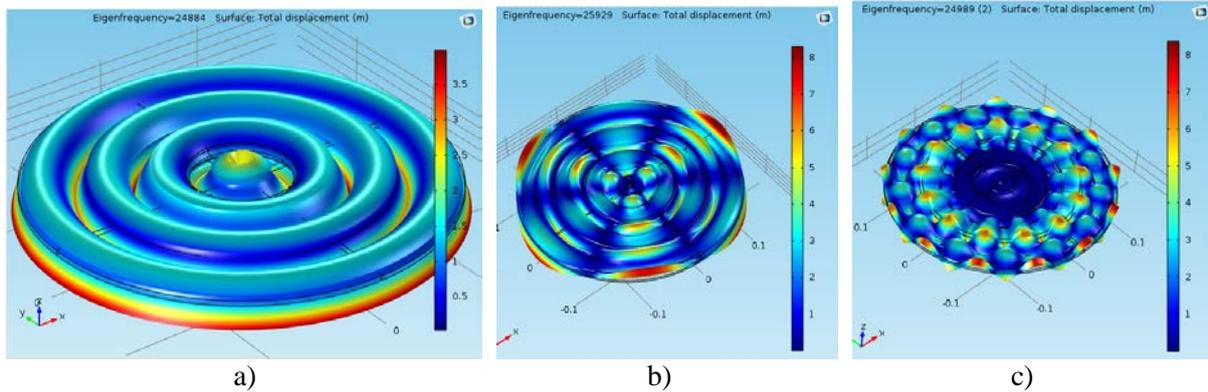
Figure 3 – Different vibration modes of the stepped circular plate. a) 7 nodal circles mode (24884 Hz). b) Combination of 7 nodal circles, 3 diameters and flexural modes (25929 Hz). c) Another combination with nodal circles, diameters and other shapes (24989 Hz).
