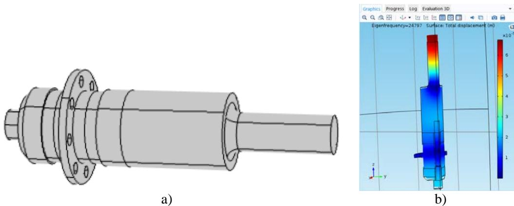
Figure 2 – Ultrasonic vibrator with sandwich and horn. a) FEM Model. b) Axial mode (24797 Hz).
