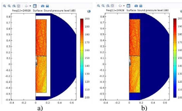
Figure 8 – Acoustic field generated inside the chamber with (a) thick or (b) thin chamber walls.
