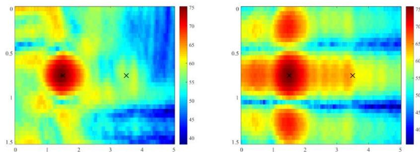
Figure 4 – Localization results of the spiral array and the separable array at 2 kHz (“x” represents the real source position and “.” represents the maximum value in the color map)
