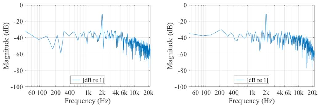
Figure 5 – Beamforming output spectra with array angle steering to the left source position (left: spiral array, right: separable array)
