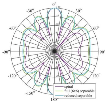
Figure 2 – The beam pattern of the three arrays
