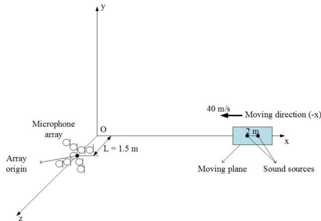
Figure 3 - Moving sound source measured by microphone array
