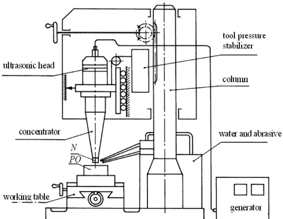
Figure. 1. Ultrasonic drill [4]
