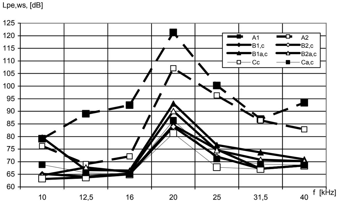
Rys. 1. Emission sound pressure level in the  $L_{pe,ws}$  1/3 octave band in case of machines :
