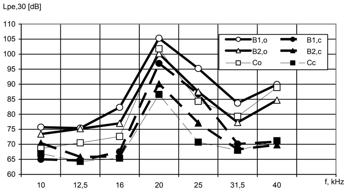
Figure 2. Emission sound pressure level in the  $L_{pe,30}$  1/3 octave band in case of machines without a ventilation hole in the housing:
