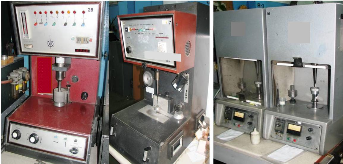
Picture 1. First type of ultrasonic drills ( $A_1$ ,  $A_2$ )
