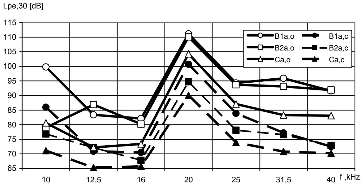
Figure 3. Emission sound pressure level in the 1/3 octave band in case of machines with a hole in the housing:
