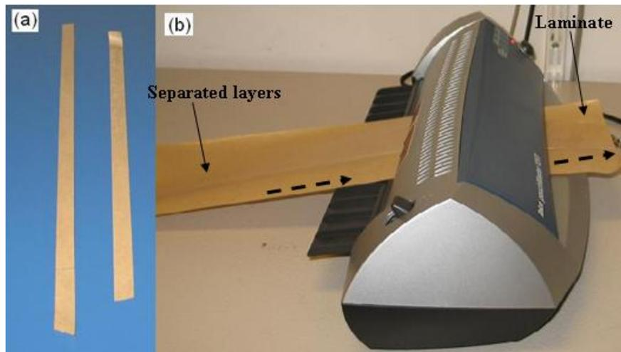
Figure 1 – Basic layers used in our tests: (a) Specimen shape; (b) Laminate preparation.
