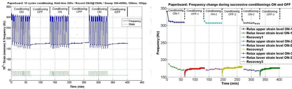
Figure 4 – Left: Conditioning strain and resonance frequency response of paperboard. The conditioning strain is alternately applied and turned off. Right: Change in resonance frequency in response to the conditioning strain of approximately  $1.6 \times 10^{-3}$ .
