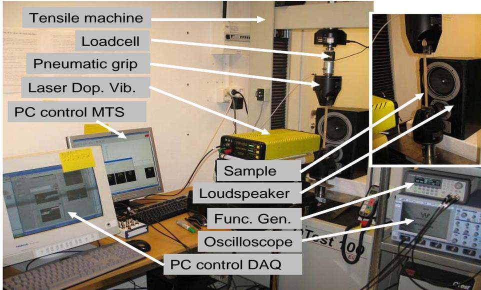
Figure 2 – Experimental setup.
