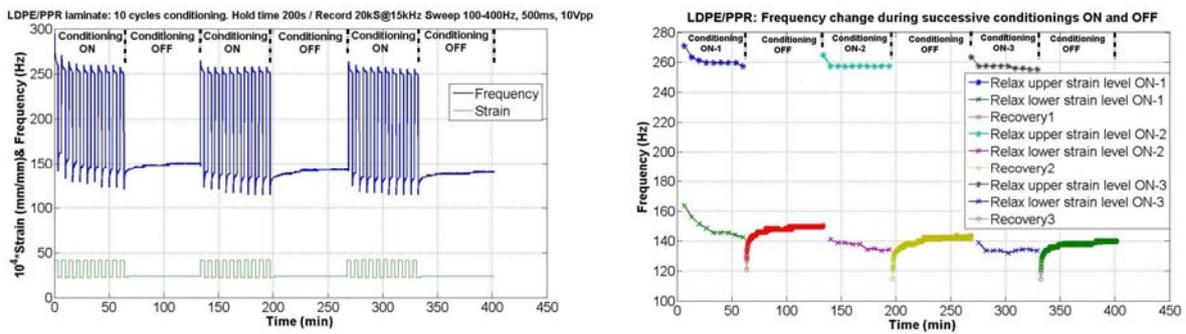
Figure 6 – Measurements on LDPE/PPR laminate. Left: Conditioning strain and response frequency. Right: Change in resonance frequency in response to a conditioning strain of approximately  $1.6 \times 10^{-3}$ .
