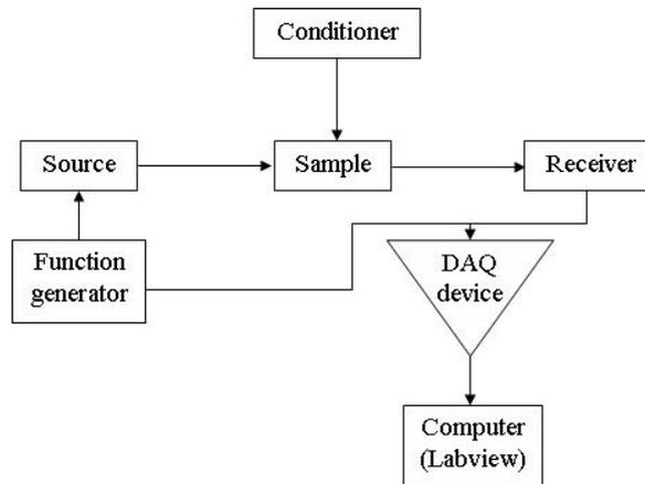
Figure 3 – Block diagram of our experimental arrangement.
