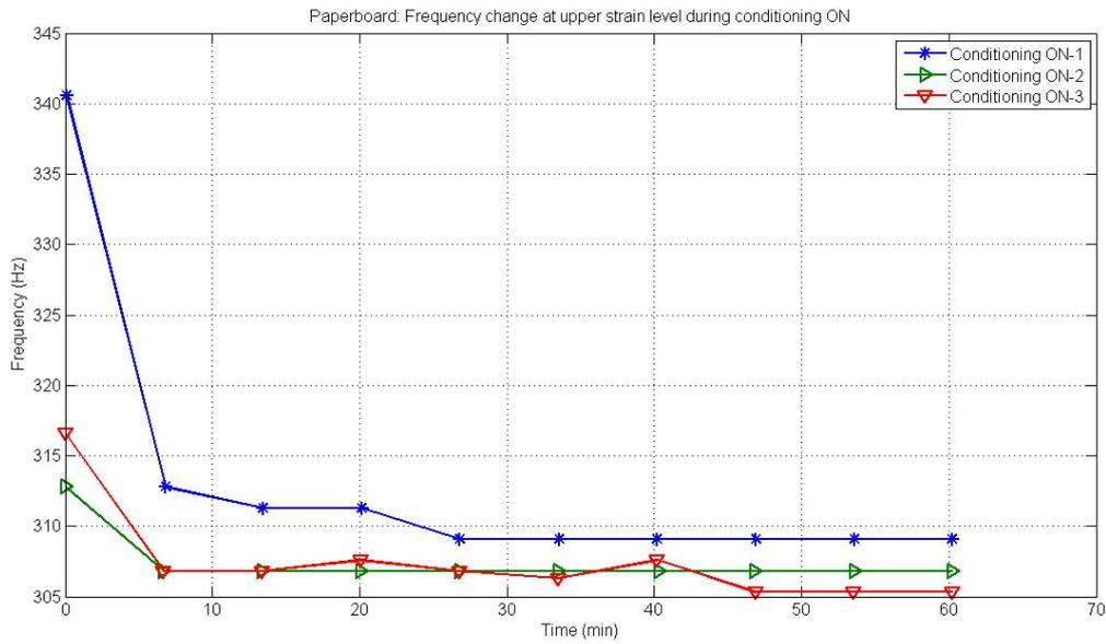
Figure 5 – Frequency change at all three conditionings ON on top of each other, monitored from upper strain level. The gap between ON-1 and ON-2/ON-3 expresses the softening of the material with total conditioning time.
