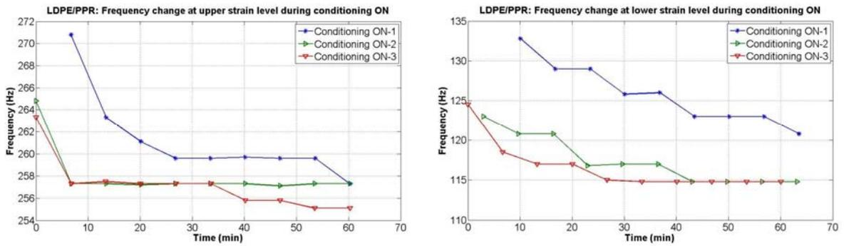
Figure 7 – Frequency change at upper (left) and lower (right) strain level for all conditionings ON, on top of each other. Increased softening is observed from ON-1 to ON-3.
