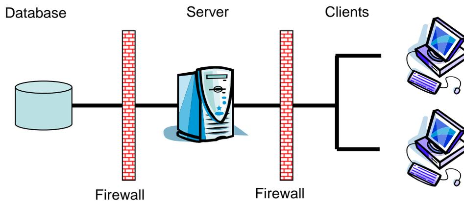
Fig. 1. Modern 3-tier client-server architecture
