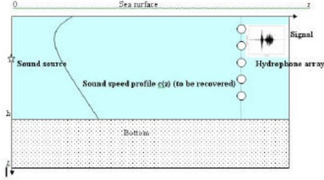
Figure 1. A typical vertical slice for ocean acoustic tomography. In the figure, the sound speed profile is considered depth dependent only (range independent environment)
