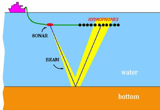
Figure 2: A typical layout of an experiment aiming at bottom classification. The inversion procedure makes use of the measurements of the acoustic field at the horizontal array of hydrophones
