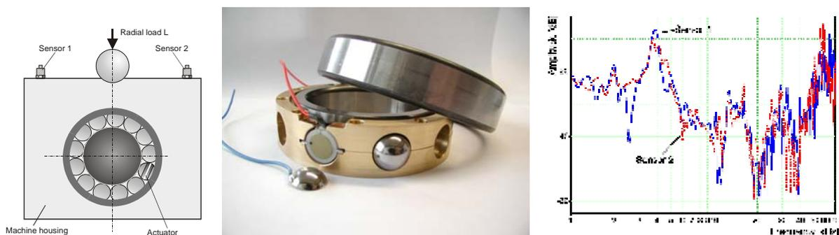
Figure 1: *Schematic positioning of sensors and actuator (left). Built in actuators of ball - detail of fixing (centre) and measured transfer function for 16 kN of radial load.*
