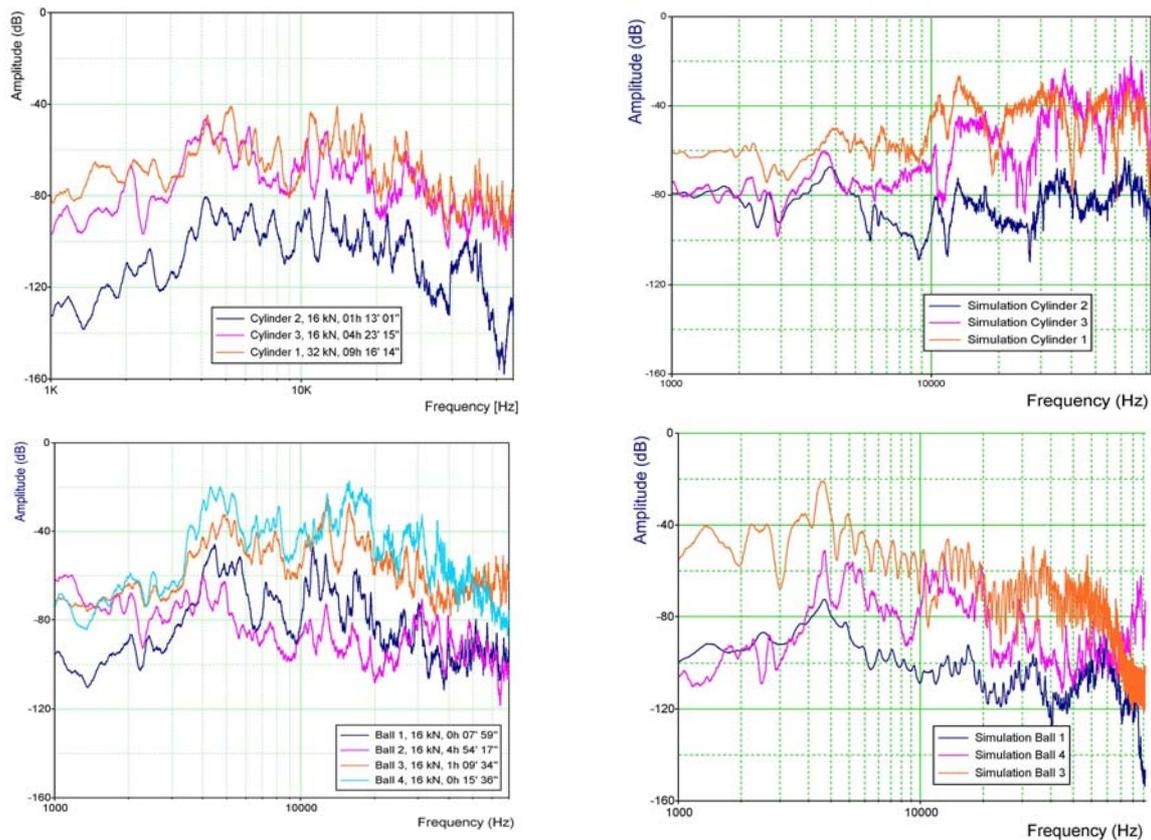
Figure 5: *Measurements (left) and simulations (right) and for 720 RPM and 16 kN radial load.*
