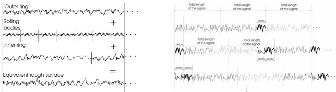
Figure 2 - Creation of the equivalent rough surface(left) and combination of the signal produced by each rolling bearing(right).
