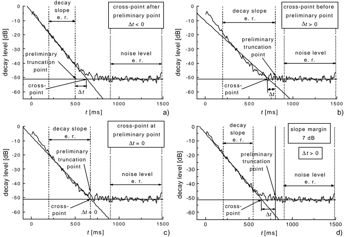
Fig. 2. Determination of truncation point by implementation of proposed algorithm a), b) and c), and modification of this procedure introducing slope and noise margin d) (e.r. is estimation range)
