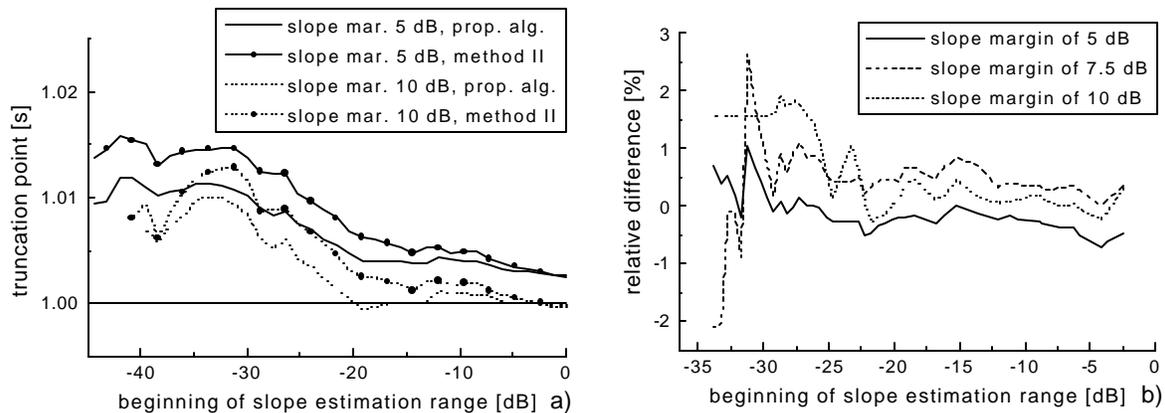
Fig. 3. The truncation points determined by proposed algorithm and method II using simulated impulse response a) and relative difference between truncation points determined by these methods using measured response b) for noise margin of 5 dB
