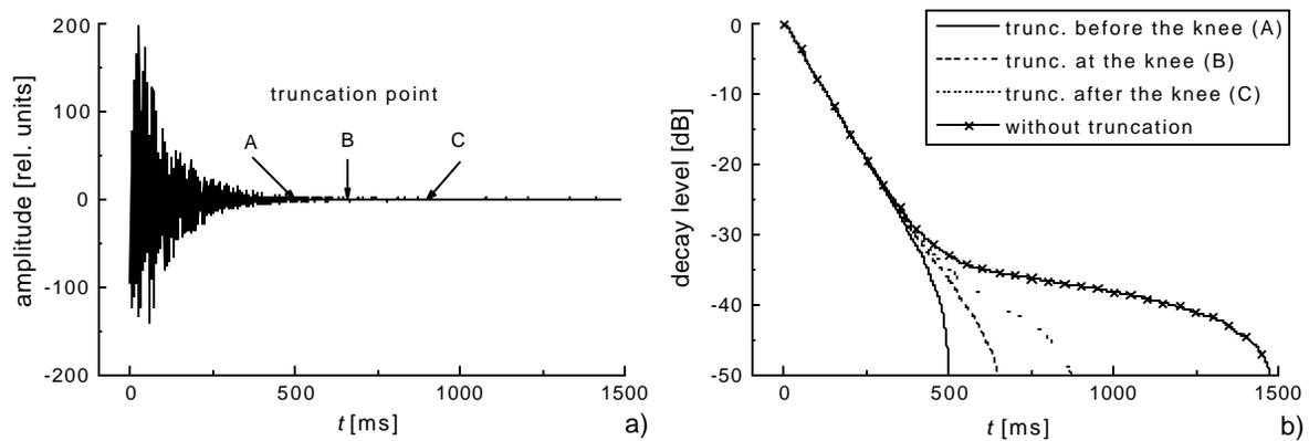
Fig. 1. Impulse response with truncation points a), and integrated impulse response obtained with and without truncation at the indicated points b)
