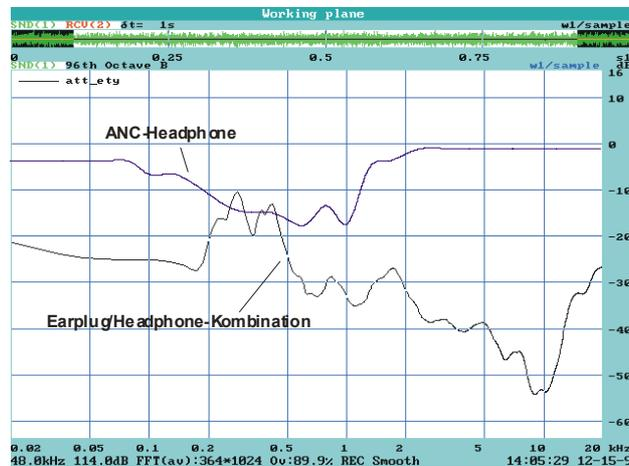
Fig.2 : Base sound reduction due to ANC headphones and earplug/headphone combination
