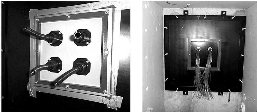
**Figure 2.** The mounting of four connectors to the test assembly (left). The test assembly seen from the source room (right).
