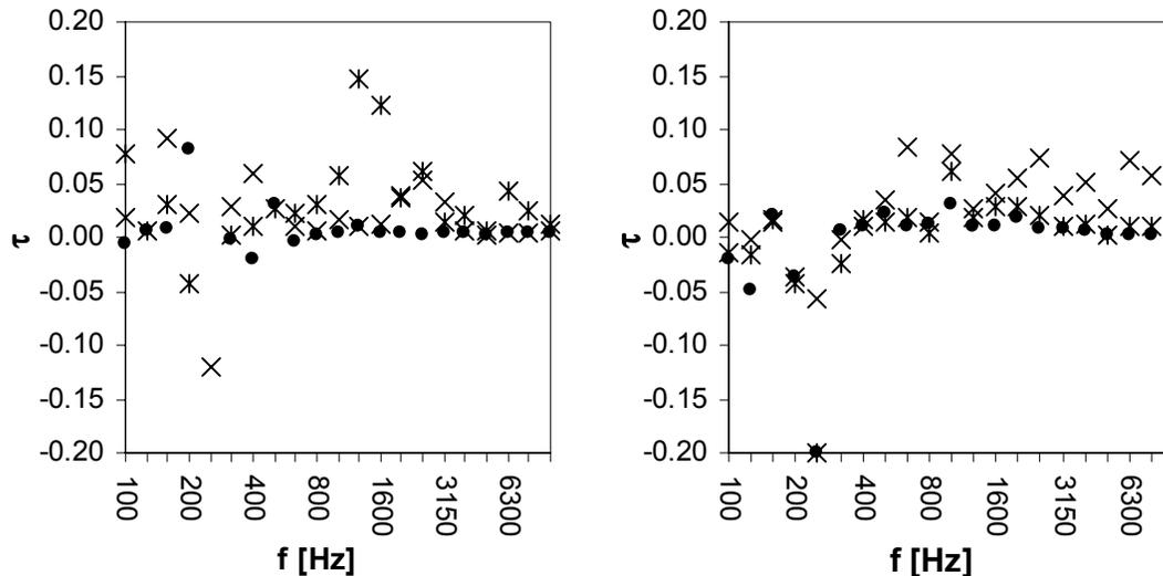
**Figure 4.** LEFT: The sound transmission coefficient of three different connectors. Key: plastic connector without sealing rubber (x), alloy connector (\*), plastic connector with rubber sealing (dot). RIGHT effect of wiring on the transmission coefficient: plastic connector, no wiring (x); half of the holes wired (\*), fully wired (dot).
