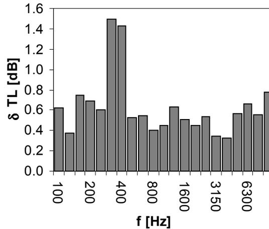
**Figure 3.** The measurement uncertainty of the system, here given as the deviation of transmission loss.
