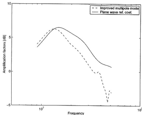
Figure 6 : Horn effect amplifications over absorbing surfaces - tyre height = 20 cm.
