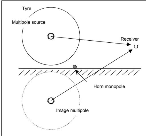
Figure 1 : Geometry of the multipole model
