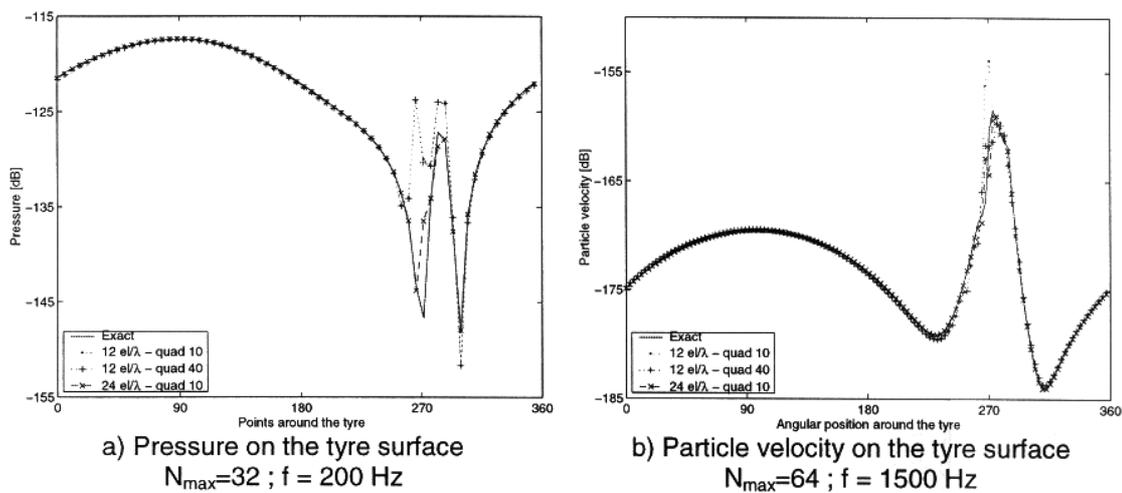
Figure 4 : Field from a vibrating tyre 1mm above a totally soft surface – tyre height = 1 mm.
