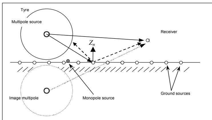
Figure 6 : Geometry of the improved multipole model.
