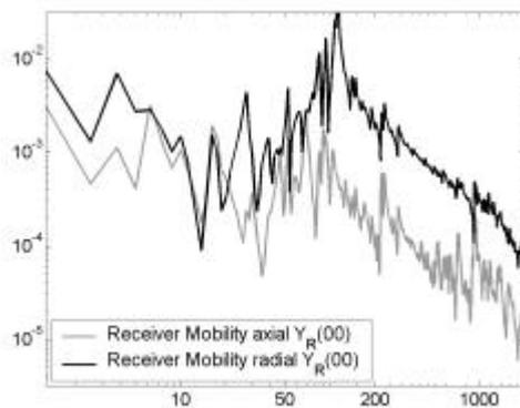
Figure 2: Magnitude of mobility of the receiving structure
