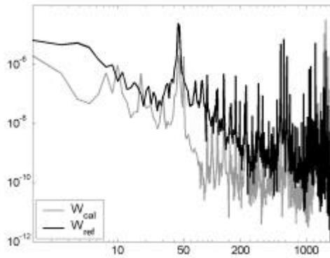
Figure 4: Comparison of the reference measurement - black - (pump mounted on the plywood plate) with the power - grey -, calculated from the mobilities of source and receiver and the free velocity
