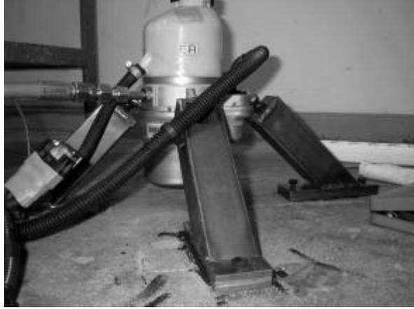
Figure 1: Servo steering pump equip with three rubber isolators mounted upon three steel stands.
