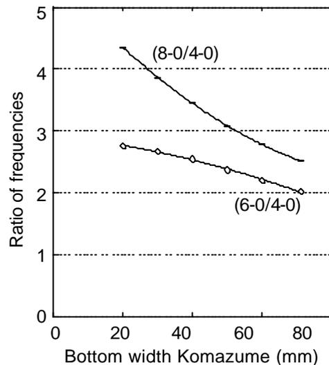
Fig. 5 Relationships between  $t_t$  values and ratios of 6-0 and 8-0 vibration mode frequencies to that of the 4-0 mode
