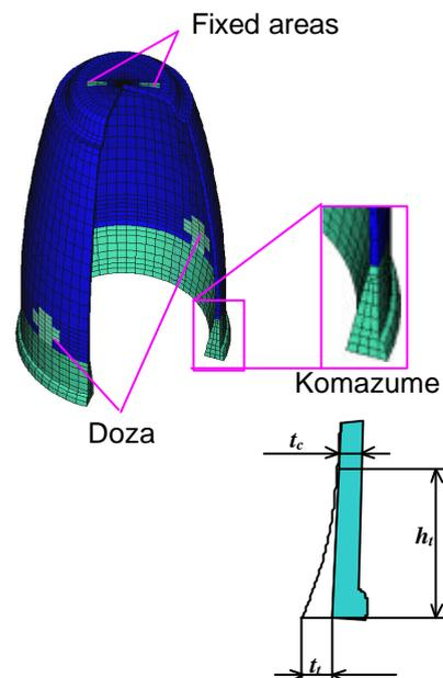
Fig.1 The FEM analysis model of the bell
