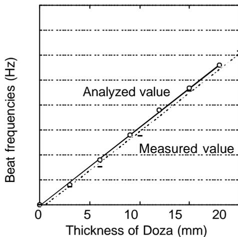
Fig.12 Experimental and simulated results showing the relationships between the thickness of Doza  $t_d$  and the beat frequencies of the miniaturized bell
