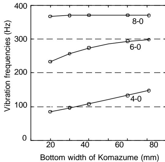
Fig.2 Relationships between three vibration mode frequencies and bottom width of Komazume  $t_b$
