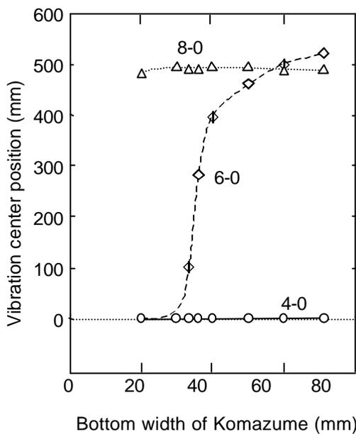
Fig.3 Relationships between vibration center positions for three vibration modes and bottom width of Komazume  $t_t$
