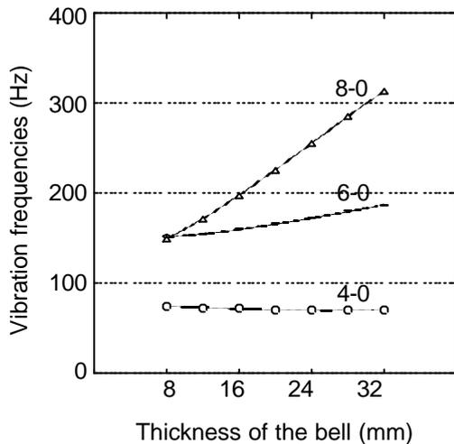
Fig.6 Influence of thickness  $t_c$  of higher bell positions on each vibration mode frequency
