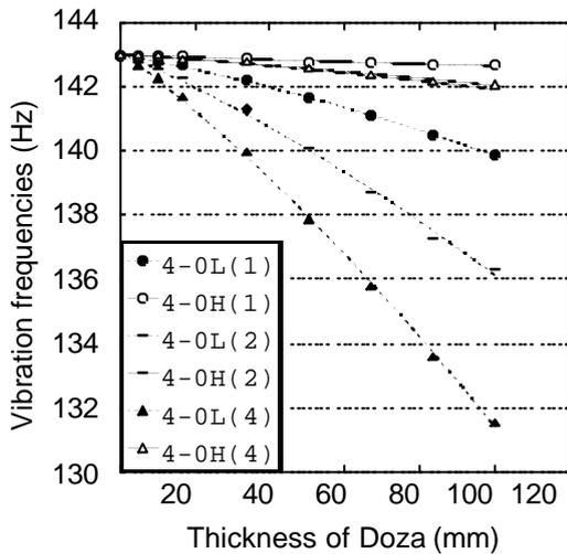
Fig.8 Relationships between 4-0H and 4-0L mode vibration frequencies and the thickness of Doza  $t_d$ , where number of Dozas are 1, 2 and 4
