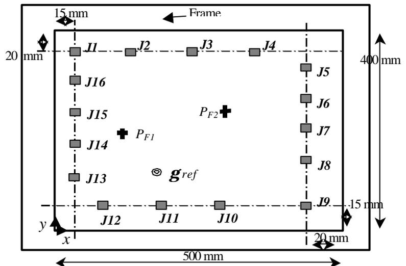
Fig. 3 : frame, plate and location of sensors ( $J1$  to  $J16$ ), excitation points ( $P_{F1}$ ,  $P_{F2}$ ) and reference sensor  $g_{ref}$
