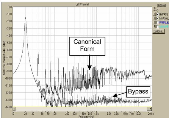
Figure 9 – Bypass of the system with 20 Hz input signal and Canonical implementation of the allpass filter degrading the signal more than 40 dB with noise and distortion.
