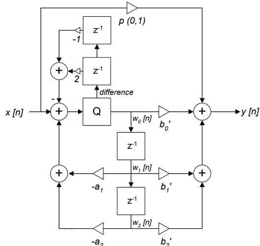
Figure 5 -  $H(z)$  with 2<sup>nd</sup> order Noise-Shaping
