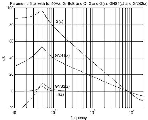
Figure 6 – Effect of Noise-Shaping
