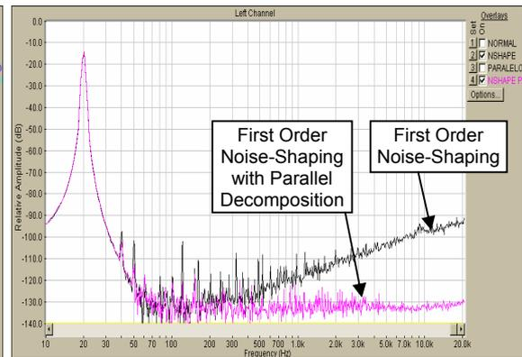
Figure 10 – Canonical implementation with First Order Noise-Shaping where the round-off noise is moved to the high frequencies, and with Parallel Decomposition, where  $H_p(z)$  (bandpass) filters this noise, obtaining the same performance than the bypass measure.
