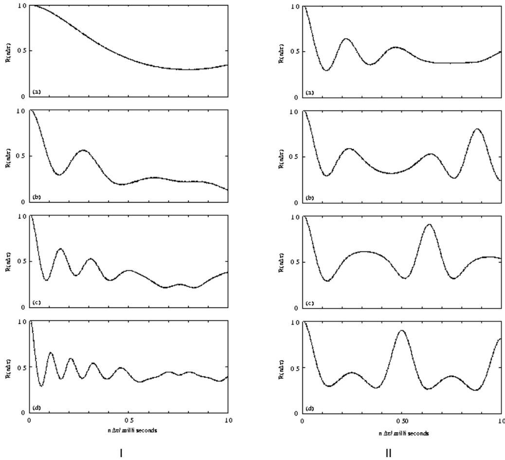
Figure 2: AutoCorrelation Functions showing effect of pressure (I) and acoustic frequency (II)
