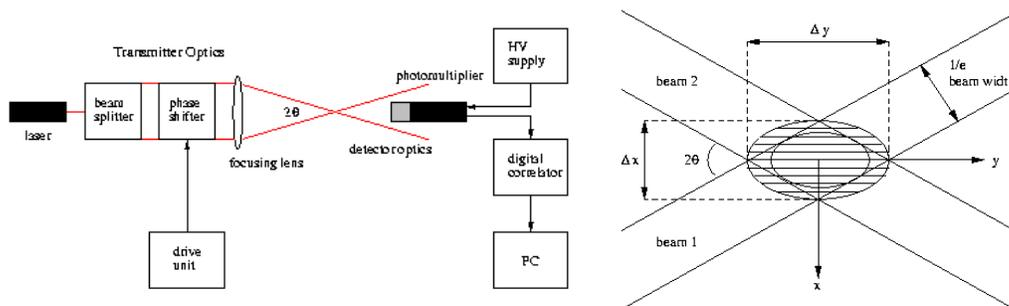
Figure 1: Photon Correlation Apparatus and Measurement Volume
