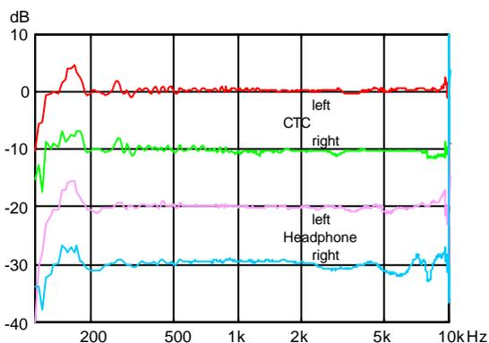
Fig. 6: Deviation of frequency response in comparison to loudspeaker reproduction.
