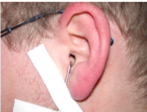
Fig. 4: Probe microphone attached to the ear
