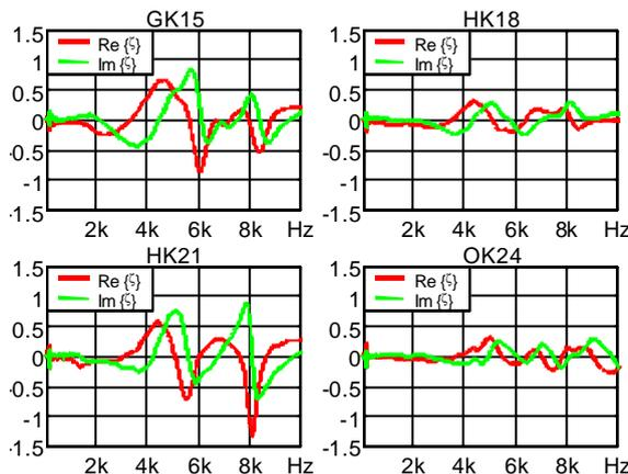
Fig. 1: Additional acoustical load on the ear of four headphones under test
