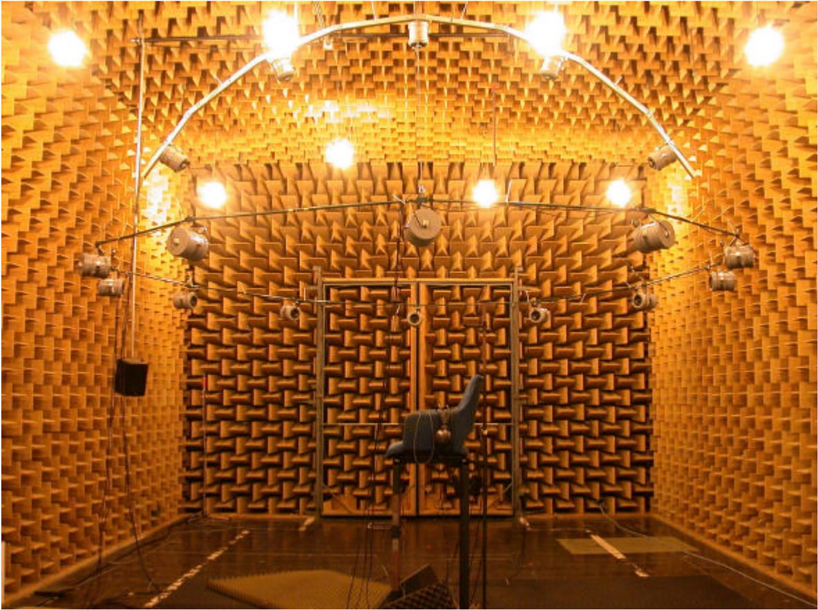
Fig. 3: Experimental setup in anechoic room
