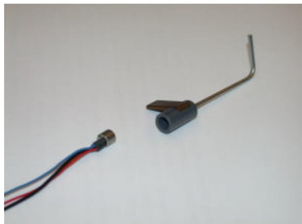
Fig. 5: Probe microphone (based on Sennheiser KE4)
