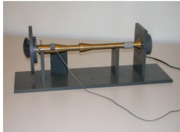
Fig. 2: Impedance tube. Note the pinna termination on the left end.
