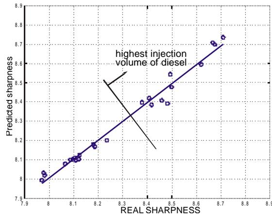
Figure 4. Predicted sharpness versus real sharpness for high r.p.m. signals.
