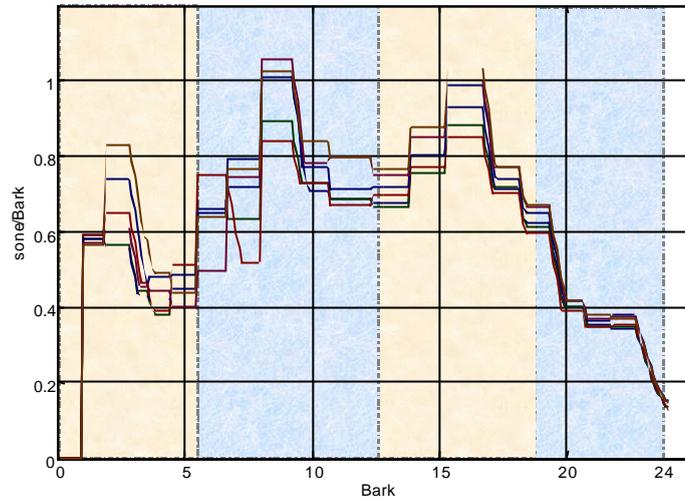
Figure 1. Stationary loudness of several noises recorded at 3000 r.p.m.
