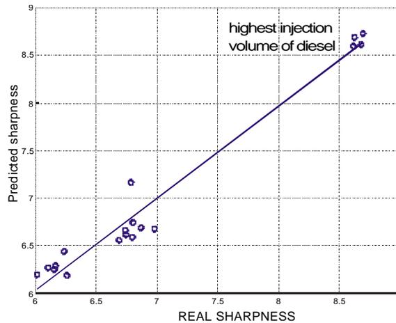
Figure 3. Predicted sharpness versus real sharpness for low r.p.m. signals.
