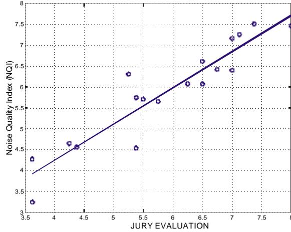
Figure 2. Noise Quality Index versus jury assessment for low r.p.m. signals.
