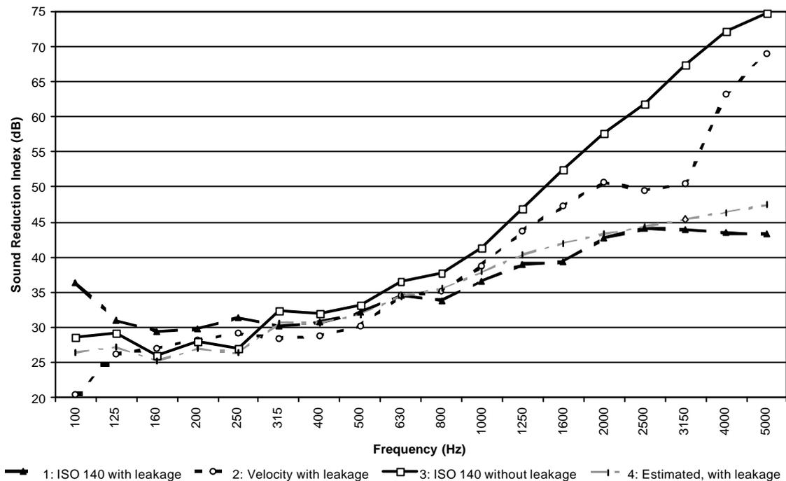
Figure 3: Sound Reduction Index of the partition with (1, 2) and without the leakage (3), measured with different techniques, and estimated (4).
