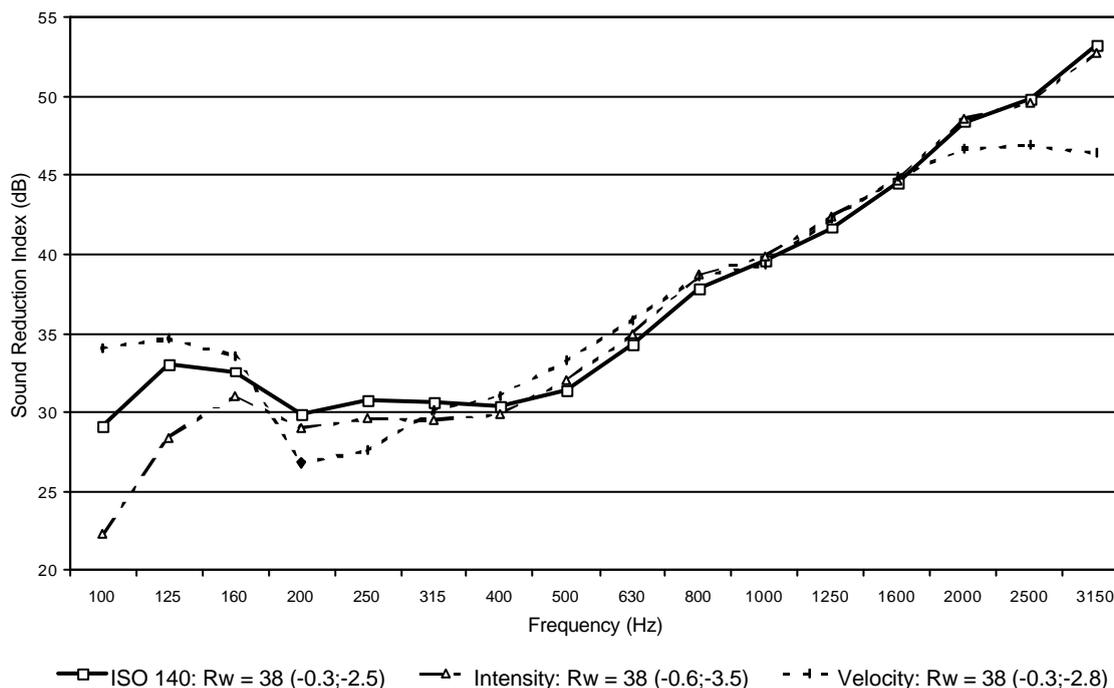
Figure 1: results of SRI measurements in the test wall, with the three techniques.
