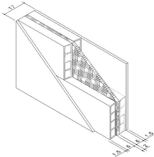
Figure 2: axonometric view of the double partition of the case study.
