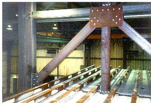
In the first set-up both floor elements were supported by one common IPE beam. Rubber plates between the floor elements and beam were applied. In this set-up, there was no 'decoupling' by the rubber due to the fact that the bending stiffness of the IPE beam was not high enough. However, from this set-up some valuable data concerning other transmission paths than the one considered in the second set-up have been measured.
