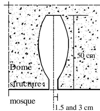
Figure 4. The cross section of the resonator at the dome of Blue Mosque
