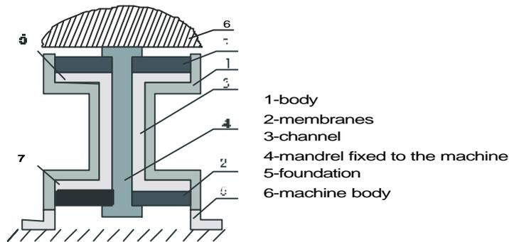
Fig.8. The diagram of the DAVI rubber-oil vibroinsulator.
