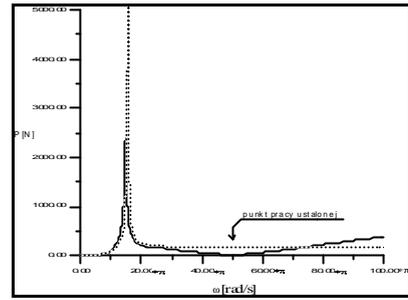
Fig. 4 The dependence of forces transmitted to the base on the forced frequency.
