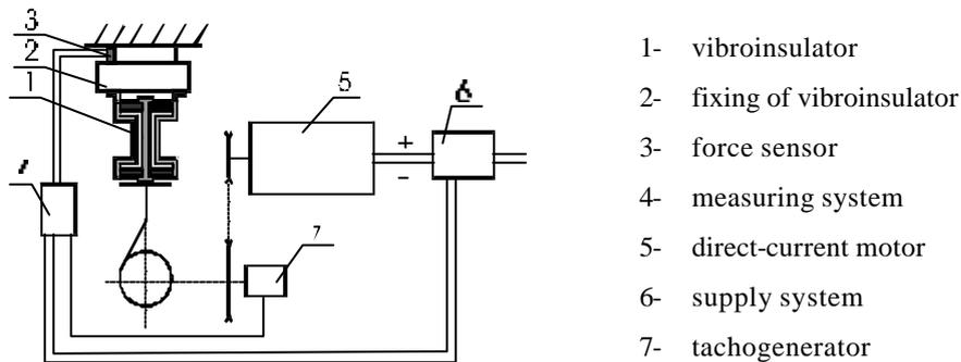
Fig. 9. The scheme of the experimental set up.
