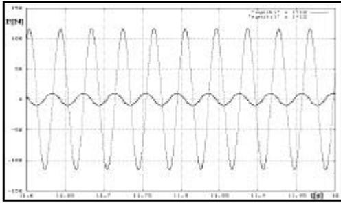
Fig. 3 Forces transmitted to the base by two types of vibroinsulation.
