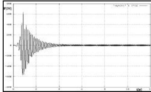
Fig. 7 Forces transmitted to the base by the system with the typical DAVI vibroinsulator
