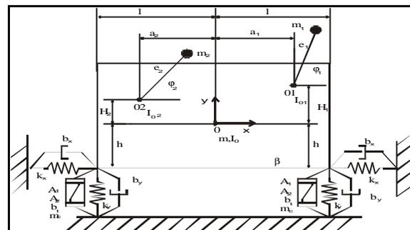
Fig. 2. The model of a vibroinsulated two-rotor machine
