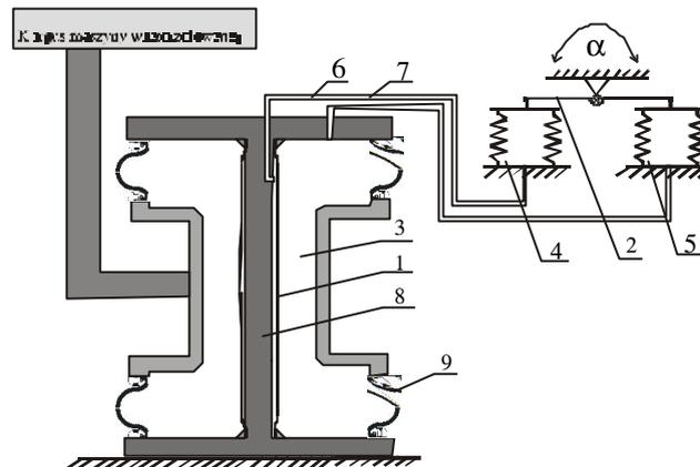
Fig. 5 Diagram of a semiactive vibroinsulator
