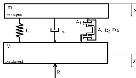
Fig.1 Analysed model of the vibroinsulating system.
