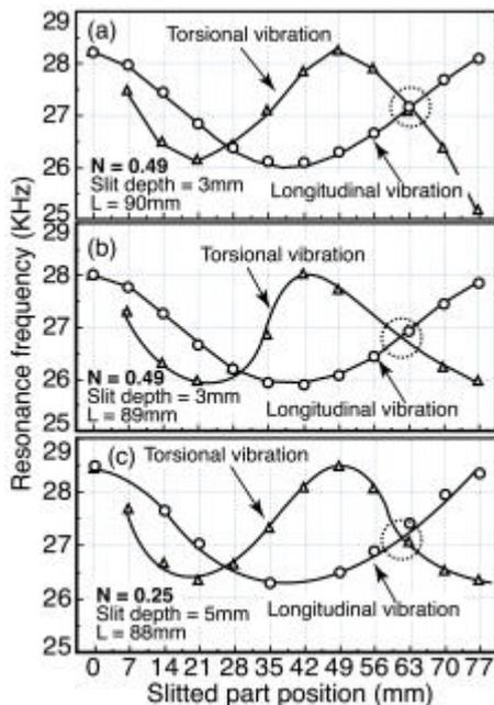
Fig.3. Relationship between slitted part position and calculated longitudinal and torsional resonance frequencies.  $N = 0.49$  and  $0.25$ .
