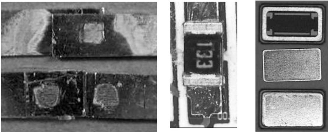
Fig. 7. Aluminum plates welded by 100 kHz. Fig. 8. Tip element. Fig. 9. Ceramic package.
