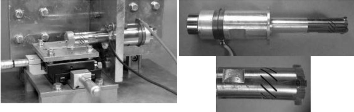
5. 40 kHz complex vibration welding system Fig. 6. 100 kHz complex vibration system and with a complex vibration converter. longitudinal-torsional vibration converter.
