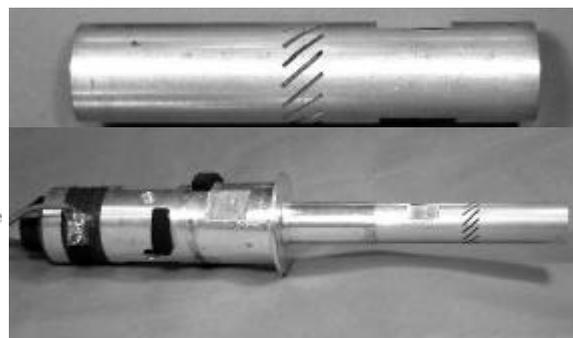
Fig.1. One-dimensional longitudinal to torsional vibration converter with diagonal slits
