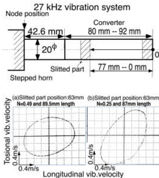
Fig.4. Vibration loci at the free edge of the converters.
