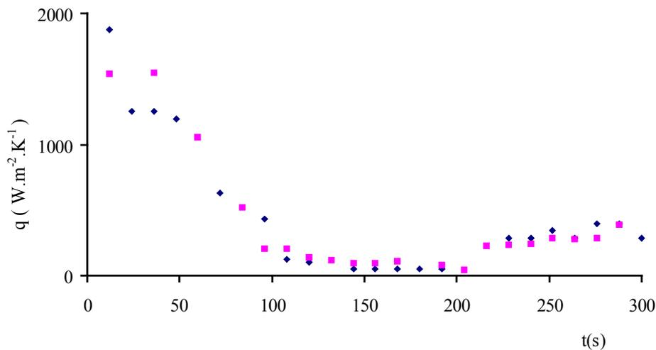
Fig. 2. The heat transfer coefficient as a function of time during solidification.
