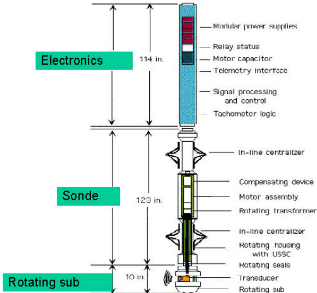
Figure 1: Schematic of the ultrasonic sonde.
