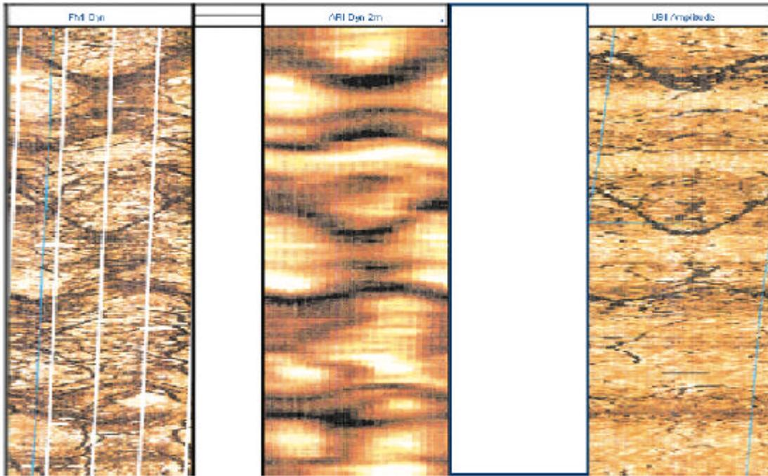
Figure 2: Example of ultrasonic amplitude image (right track) compared with high and low resolution resistivity images (left and center track). Vertical distance 13m.
