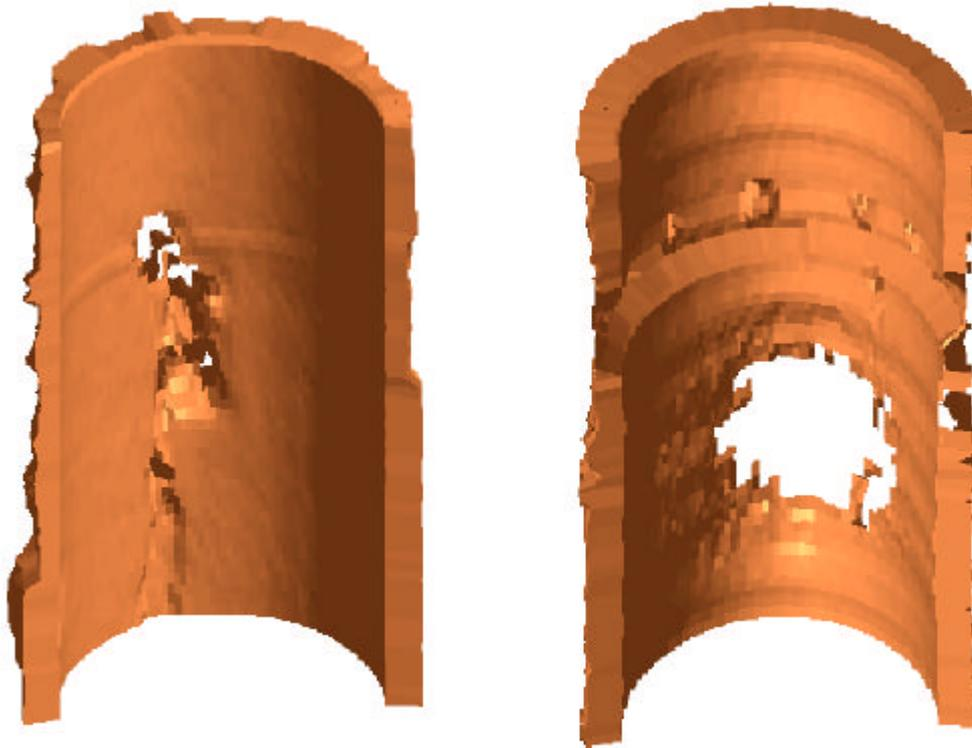
*Figure 5: 3D images of short pipe sections from ultrasonic measurement of inner radius and thickness.*
